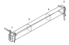
Fig. 10 Measuring the original beam section at four places
