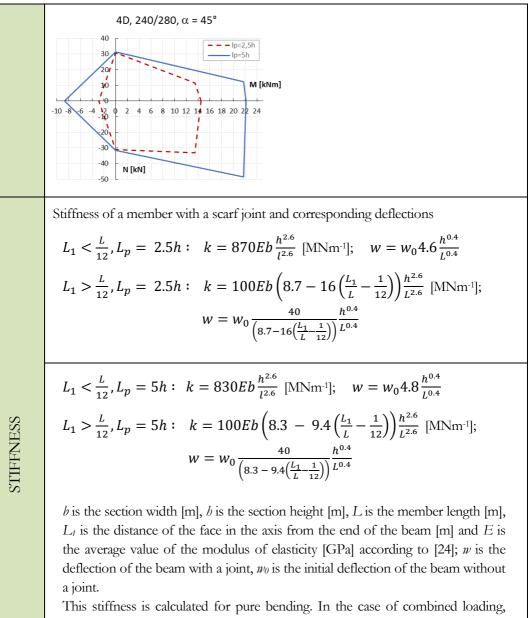
compression and bending the stiffness remains or slightly increase; in the case of tension and bending, on the other hand, the stiffness is about a quarter lower, therefore the deflection is up to a quarter higher compared to the aforementioned relations.
