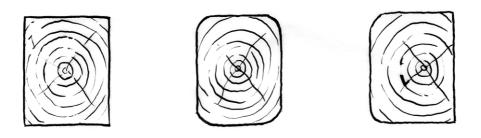
Fig. 12 a) Centric sharp-squared section, b) centric section with wanes, c) eccentric section with wanes on one side of the member
