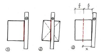
Fig. 17 Exact method of beam section measurement; 1 - determining the inclination in the middle of beam, 2 - plotting the axis of the cut on the cut off face, 3 - location of the point of the second division point at the end of the scarf joint
