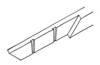
Fig. 28 Scarf joint after cleaning the grooves for keys
