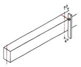
Fig. 20 Transferring the end point using a spirit level
