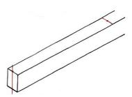
Fig. 19 Plotting the rough length of the scarf joint and marking the end point of the top surface
