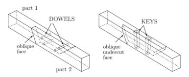
Fig. 6 Scarf joint with four dowels and scarf joint with two keys
