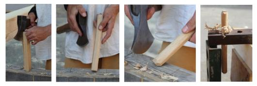
Fig. 15 Process of dowel manufacture
