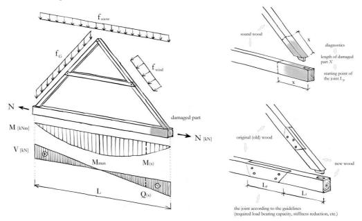
Fig. 1 Truss with damaged elements and the course of repair
