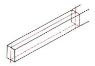
Fig. 21 Connecting points on the surfaces using a chalk line
