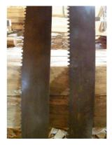
Fig. 39 Saw band for longitudinal cutting (left), saws band for cross cutting (right)
