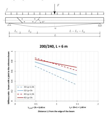
Fig. 9 Dimensions of structure and beam deflection (above), dependence of beam stiffness with a joint shifting along the beam centreline (bottom)
