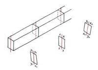
Fig. 18 Dividing the beam section into two equal halves taking into account possible twisting
