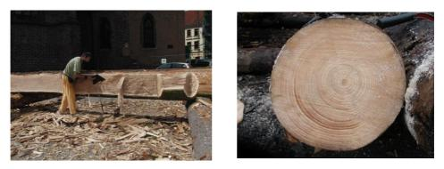
Fig. 42 Fine heaving (left), compression wood of spruce (right)
