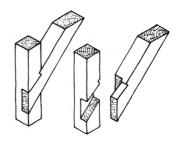
Fig. 5 Dovetail lap joint [2], [50]
