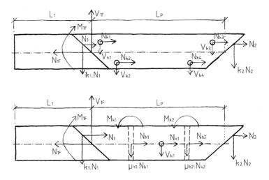
Fig. 7 Forces acting in the joint with four dowels 4D (top) and in the joint with two keys and one dowel 2K+1D (bottom).
