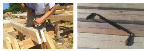
Fig. 38 Chisel axe (left), drawknife (right)
