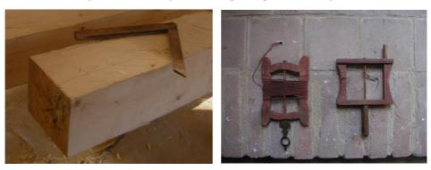
Fig. 40 Bevel gauge (left), chalk line with clay (right)
