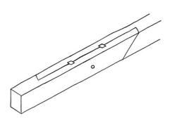
Fig. 35 Coarsely cut off coupling elements after joint assembly
