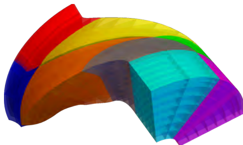
Figure 1: Part of multipatch conforming mesh of flow region in the runner wheel domain.
