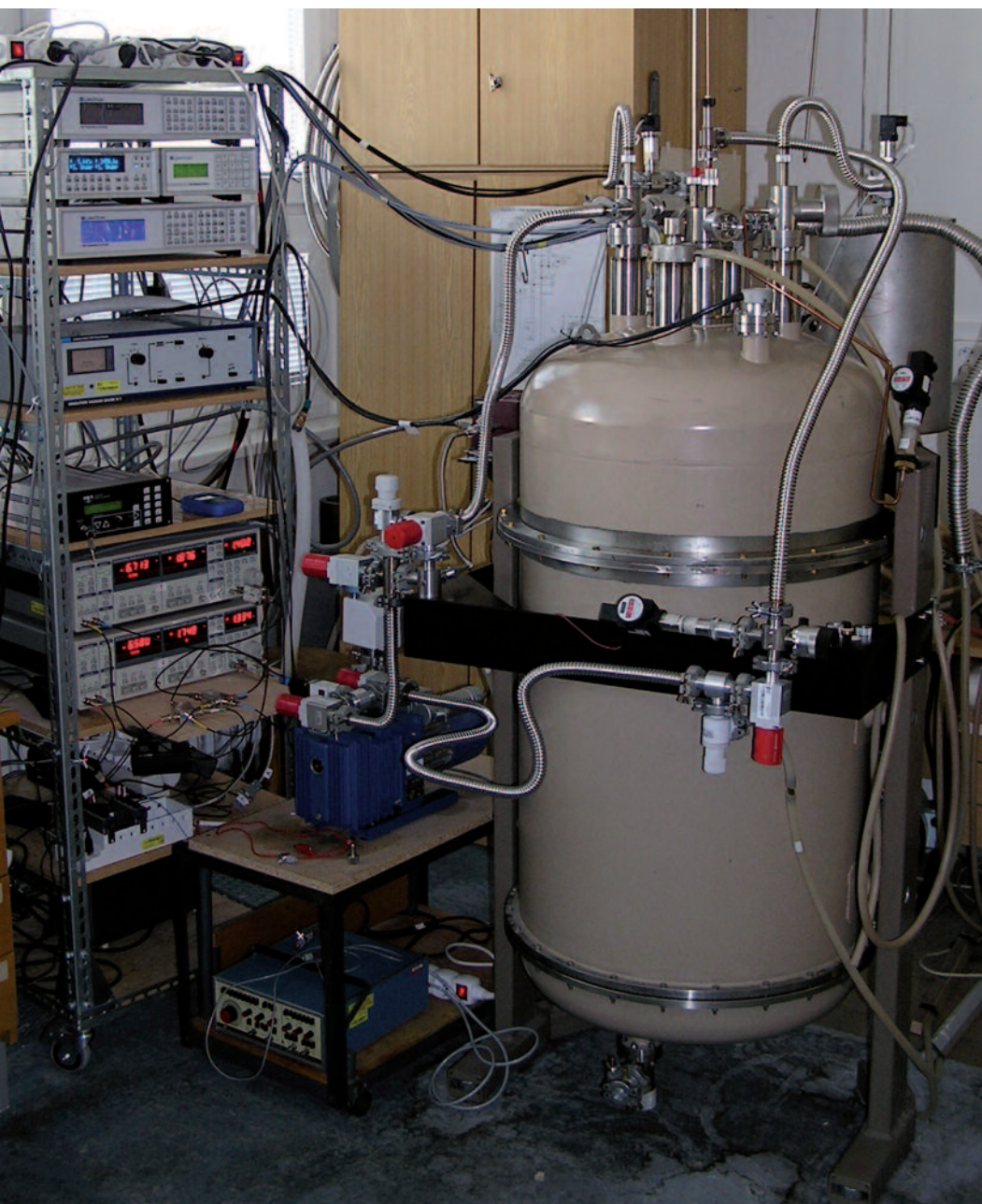
Cryostat for study of natural convection in cold helium gas
