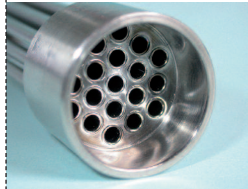
Heat exchanger welded by electron beam
