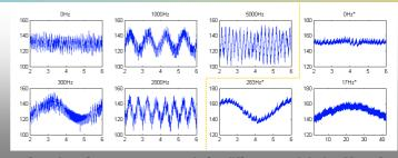
Samples of arc current records for different modulation [A; ms]
