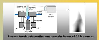
Plasma jet is generated by the experimental vertically oriented plasma torch device at atmospheric pressure. We use argon as the working gas and switching power supply as the current source.
