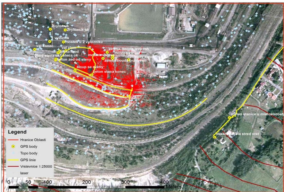
Spatial data from digital thematic maps, D-GPS, geodetic survey and laser scanning in the environment of GIS for construction of the DTM
