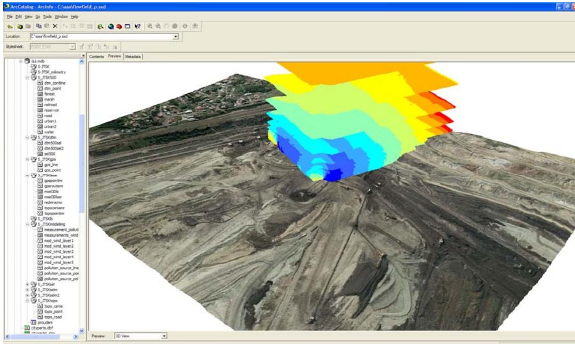
Display of simulation outputs in the environment of ArcGIS-ArcCatalog (structure of spatial data in the ArcGIS-geodatabase on the left part, a view of the simulation outputs above the aerial image draped on the DTM on the right part)
