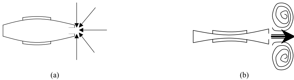
Fig.1: Schematic diagram showing the operating principle of cavity-based piezoelectric fluidic actuator.(a) Suction stage (b) blowing stage [7].
