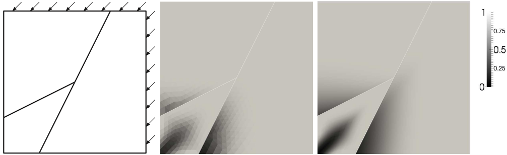
Figure 1: Transport in 2D fractured domain: geometry and direction of advection; FV solution at t = 0.18 ( \tau = 4 \cdot 10^{-4} ); DG solution at t = 0.18 ( \tau = 10^{-2} ).
