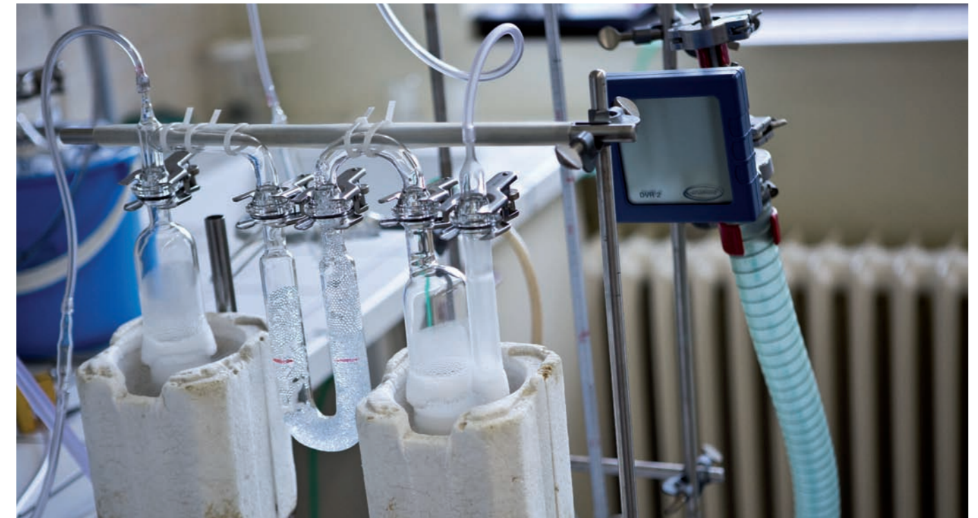
Transfer of C-14 to a chemical form suitable for the measurement of activity
