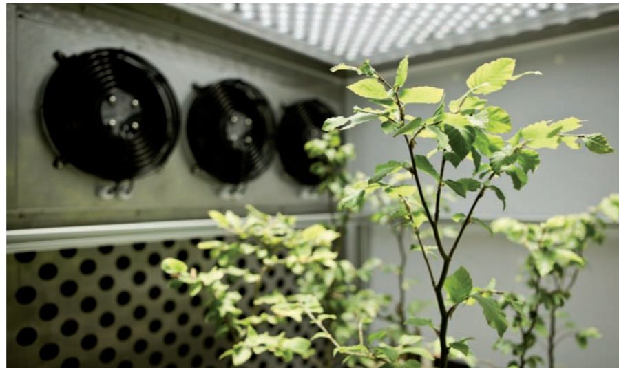
Growth chambers used for experiments to evaluate the impacts of global change allow, apart from controlling basic parameters such as air temperature or humidity, also the carbon dioxide concentration or spectral composition of light to be changed
