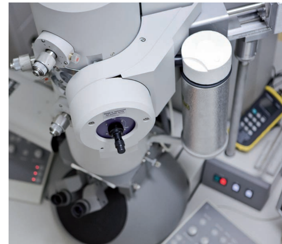
A transmission electron microscope for cryoscopic measurements
