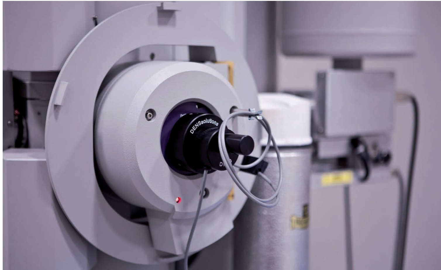
A detail of a high-resolution transmission electron microscope (HR TEM)
