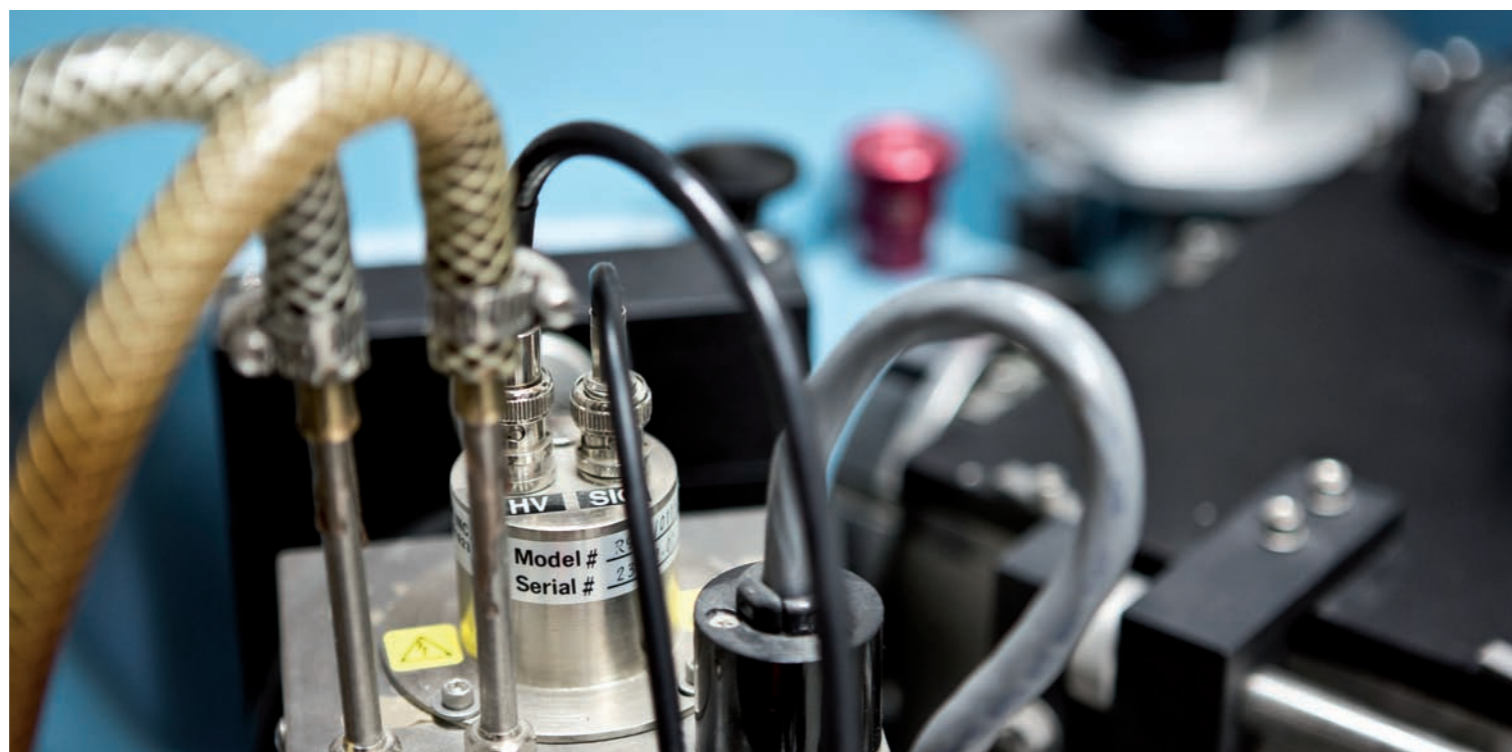
A detection unit in a McPherson VUV spectrophotometer
