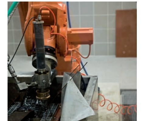
The ABB robot whilst manipulating the generator of a pulsating water jet
