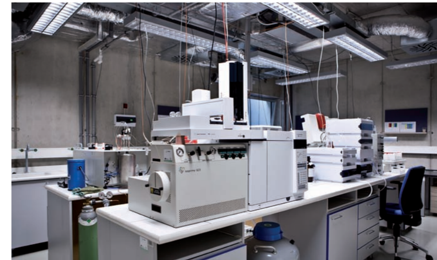
The isotopic laboratory is used to evaluate the natural discrimination of the stable isotopes of C, N, H, O, which is, for example, an indicator of the efficiency of utilisation of water by plants, or a type of photosynthetic metabolism
