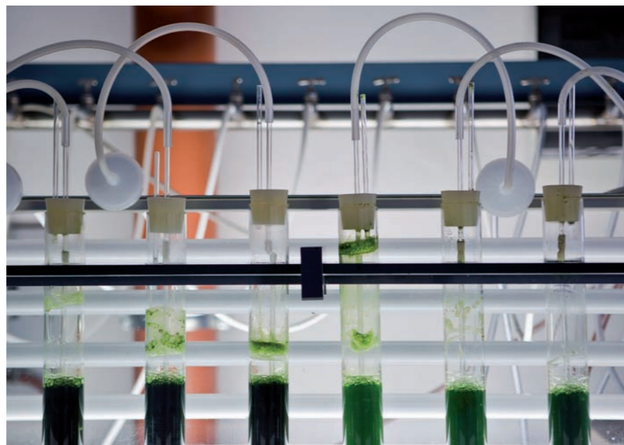
Waste-free technology of utilising recycled water for the growth of microalgae
