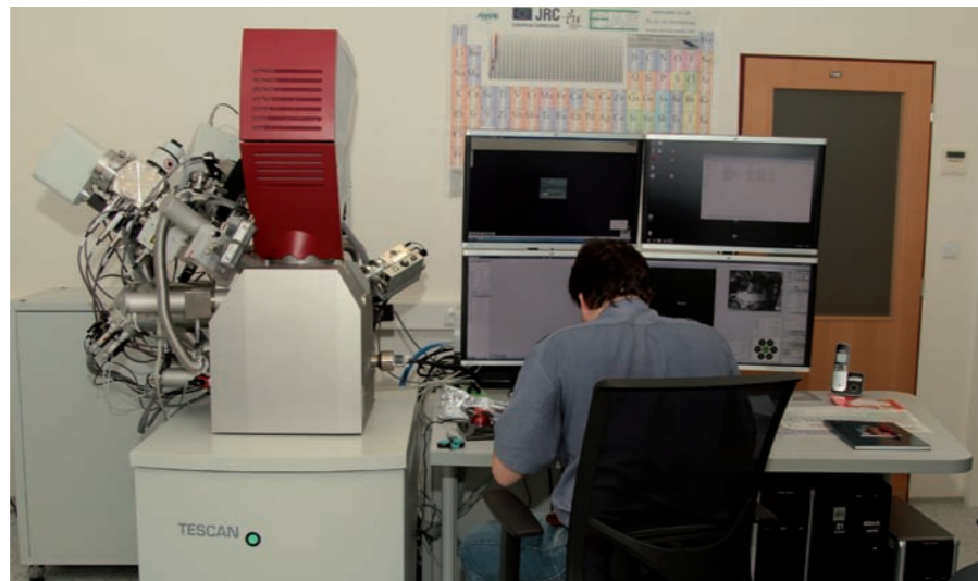
The TESCAN Fera3 scanning electron microscope with a focused ion beam for analysing the surfaces and microstructures of functional materials
