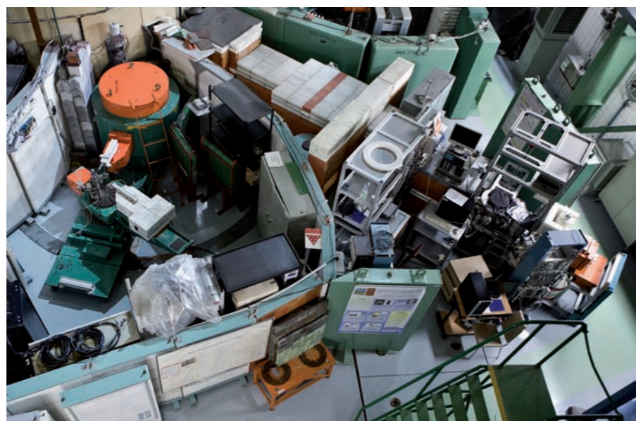
An SPN-100 neutron diffractometer for scanning tension in materials (left) and analytical methods for neutron in-depth profiling and prompt gamma activation analysis (right) on neutron beams in a research reactor
