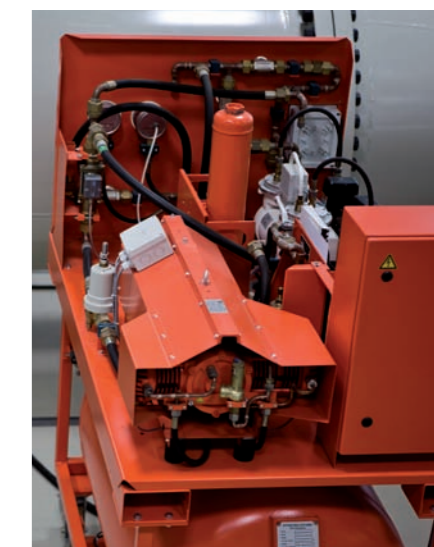
A pumping and storage vessel for the SF 6 insulation gas, whereby the acceleration part with high voltage is pressurised
