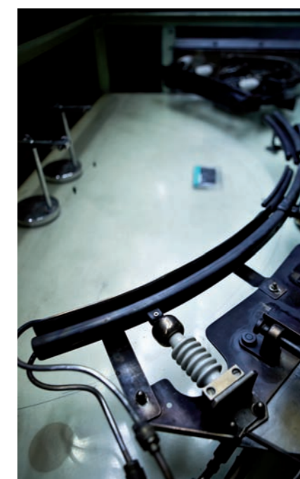
A deflection system for taking positive ions out of the cyclotron
