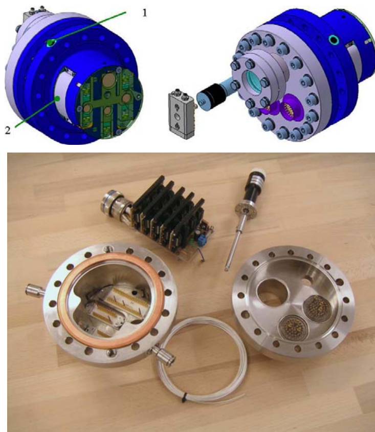
Fig. 2: Design of the port plug (top): vacuum side (left) with cooling channel (1) and mounting hole (2), atmospheric side (right). Partially assembled manufactured parts of the port plug and amplifiers (bottom).
