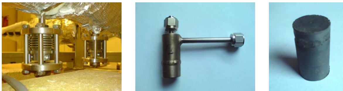
Fig. 2. Original “once shot” sampling system and new simplified one for repeatable use. Sample of PbLi.
