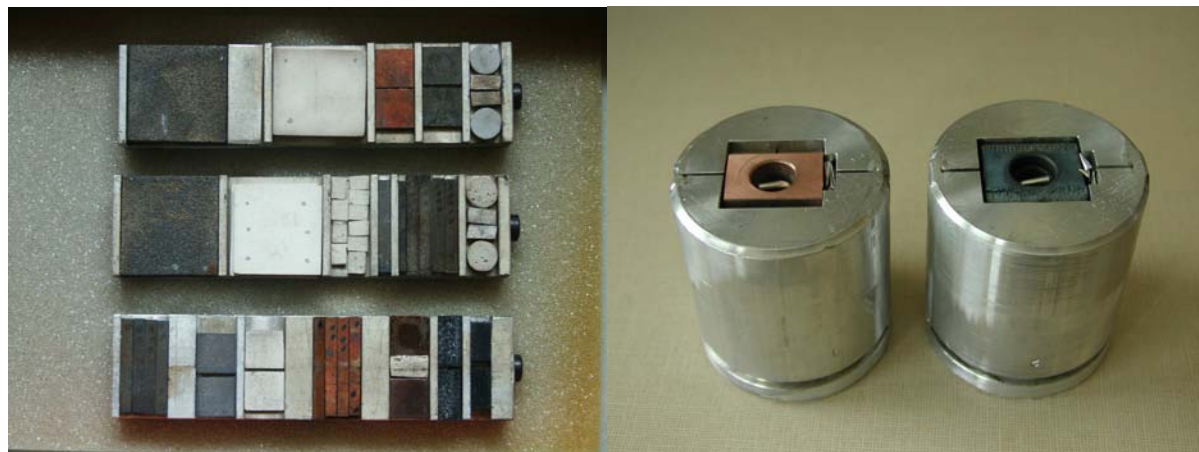
Fig. 2. L: Irradiation capsule inserts containing small samples for structural studies and measurement of thermal and electrical properties, R: capsules containing the mock-ups shown in Fig. 1. for high heat flux testing.
