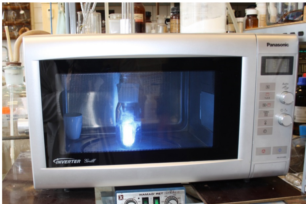
Experimental set-up for microwave photochemical experiments with EDLs
