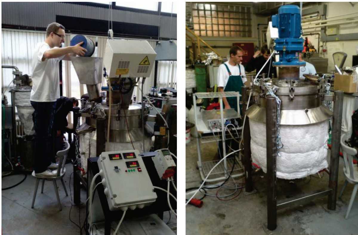
Pilot equipment for microwave thermal desorption (Dekonta a.s.)
