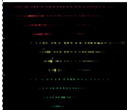
An example of optically self-arranged colloidal waveguide. The distance between the particles is tuneable by the width of two counter-propagating beams which is followed with different spectral properties of the whole structure shown at red, yellow and green wavelengths.
