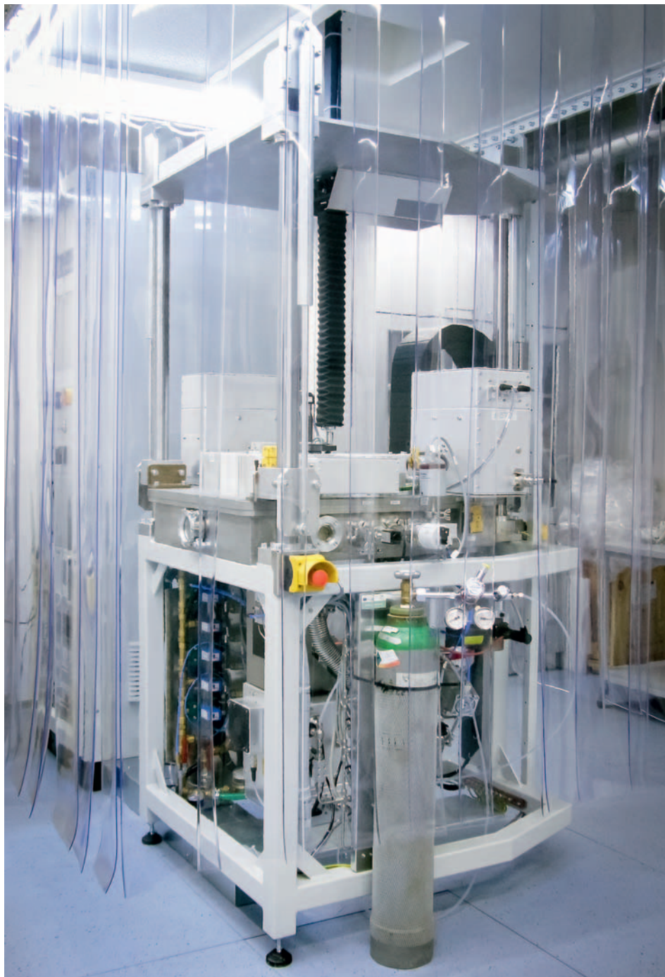
Computer controlled magnetron sputtering system Aurion
