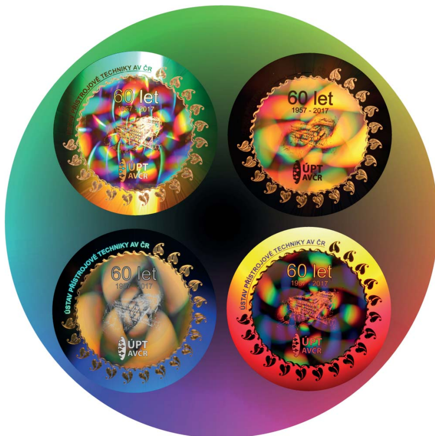
ISI in 60 years and 4 seasons Diffractive optically variable image device based on a patented approach taking advantage of spiral cross grating arrangements (quasiperiodic phyllotaxy model). The device is captured at four different lighting conditions demonstrating its outstanding potential of image variability.
