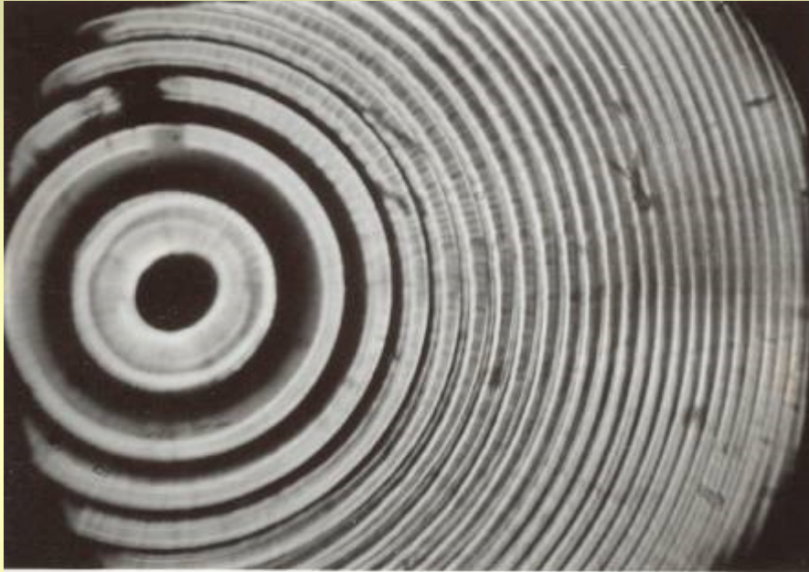
Microphoto of cross section of produced preform
