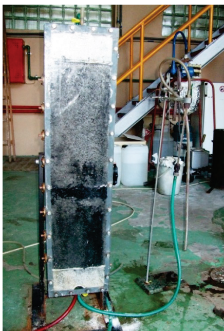
Pilot reactor with reactive barrier made by active carbon after 5 days processing
