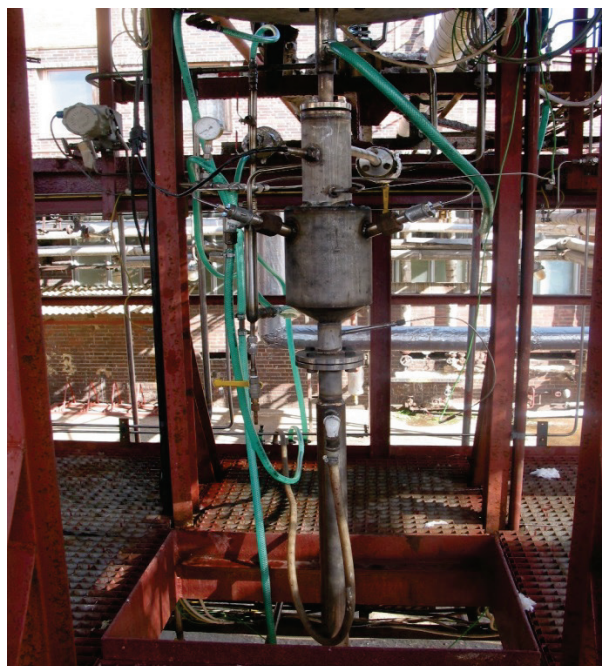
Quench of the POX reactor
