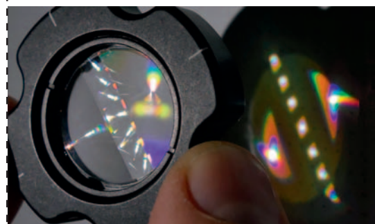
Multi-axial diffractive zonal lens
