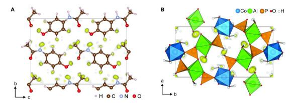
**Figure "TZ\_Science\_vodiky\_A.png" & figure ""TZ\_Science\_vodiky\_B.png":** Structure of (A) paracetamol form II and (B) cobalt aluminophosphate with superimposed difference electrostatic potential (gray and yellow isosurfaces). The maxima of the potential correspond to the positions of hydrogen atoms.
