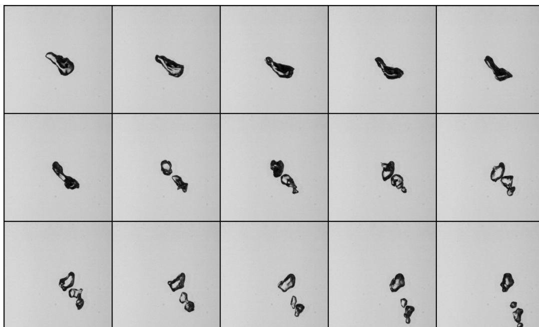
Visualization of break-up sequence of a bubble in an experimental turbulent channel
