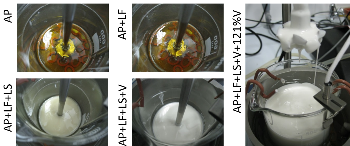
Emulsification progress with and without special additives
