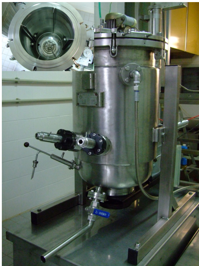
The newly designed mixotrophy reactor
