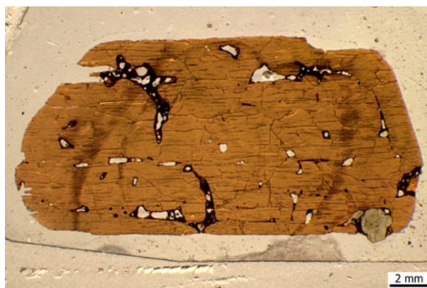
■ Fig. 19. Optical photomicrograph of a homogeneous kaersutite megacryst weathered from altered analcimite from Kostomlaty pod Milešovkou. The inclusion in the lower right part of the megacryst is of diopside composition. Photo by L. Krmiček.
