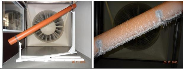
Frame construction including model fragment of cable cover suspension bridge in climatic section and the test result of the ice accretion
