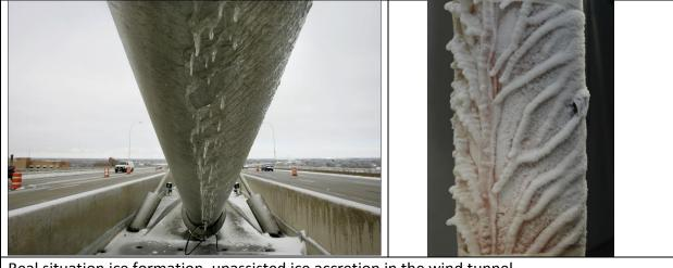
Real situation ice formation, unassisted ice accretion in the wind tunnel
