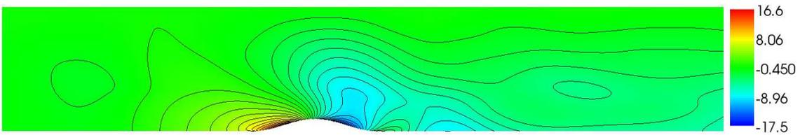
Figure 7: "Sinus hill 10%" - incompressible viscous turbulent stratified flow,  $Re = 5 \cdot 10^8$ ,  $u_\infty = 7.5 m \cdot s^{-1}$ , contours of pressure disturbances [ $pa$ ]
