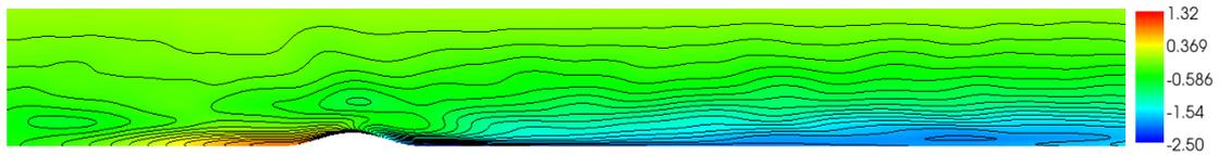
Figure 4: "Sinus hill 10%" - incompressible viscous turbulent stratified flow,  $Re = 10^8$ ,  $u_\infty = 1.5 m \cdot s^{-1}$ , contours of pressure disturbances [ $pa$ ]
