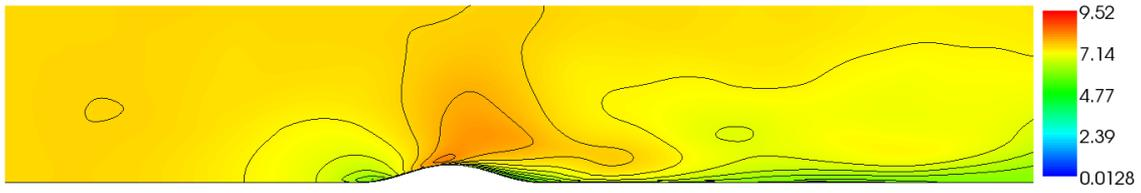
Figure 6: "Sinus hill 10%" - incompressible viscous turbulent stratified flow,  $Re = 5 \cdot 10^8$ ,  $u_\infty = 7.5 m \cdot s^{-1}$ , contours of velocity magnitude [ $m \cdot s^{-1}$ ]
