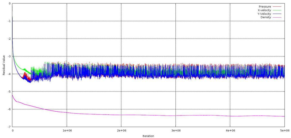
Figure 8: "Sinus hill 10%" - incompressible viscous turbulent stratified flow,  $Re = 5 \cdot 10^8$ ,  $u_\infty = 7.5 m \cdot s^{-1}$ , Residuals
