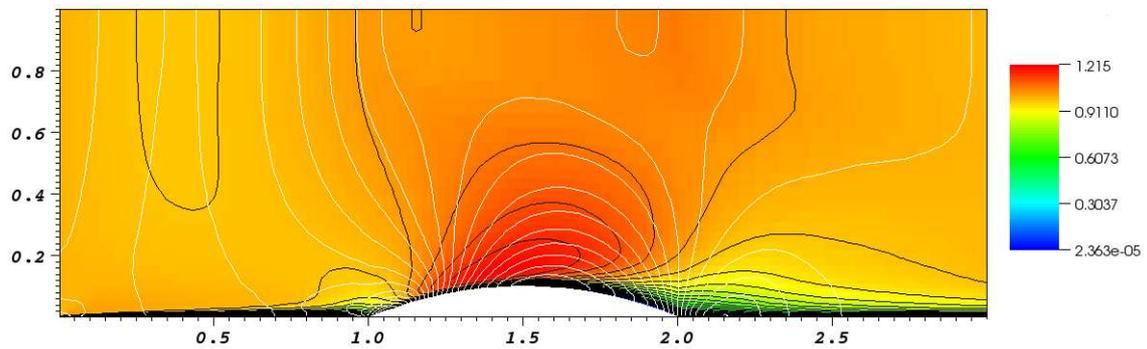
Figure 1: DCA 10% - incompressible viscous laminar flow,  $Re = 10^5$ ,  $u_\infty = 1.0$ , white lines - contours of pressure, black lines - contours of velocity magnitude
