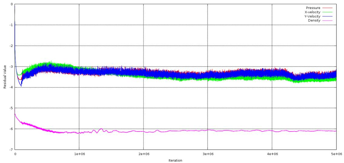
Figure 5: "Sinus hill 10%" - incompressible viscous turbulent stratified flow,  $Re = 10^8$ ,  $u_\infty = 1.5 m \cdot s^{-1}$ , Residuals
