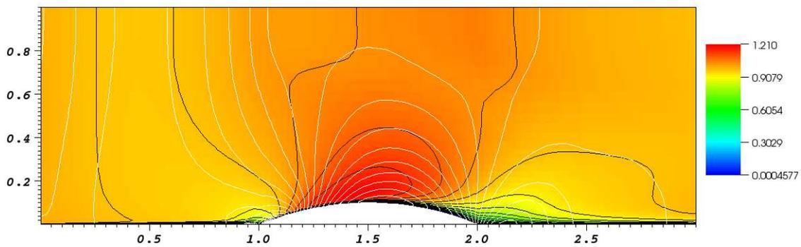
Figure 2: DCA 10% - incompressible viscous laminar flow,  $Re = 10^6$ ,  $u_\infty = 1.0$ , white lines - contours of pressure, black lines - contours of velocity magnitude
