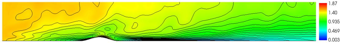
Figure 3: "Sinus hill 10%" - incompressible viscous turbulent stratified flow,  $Re = 10^8$ ,  $u_\infty = 1.5 m \cdot s^{-1}$ , contours of velocity magnitude [ $m \cdot s^{-1}$ ]
