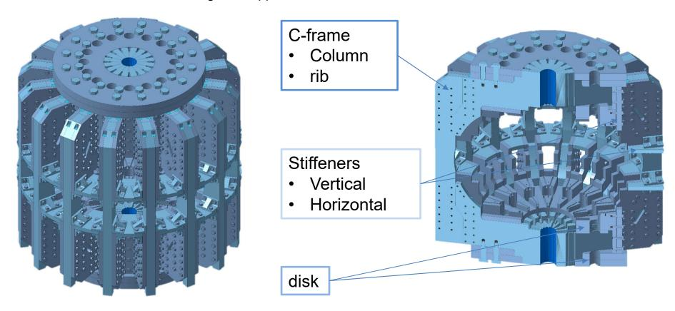
COMPASS-U support structure is under design process and can be modified later as per design requirements
