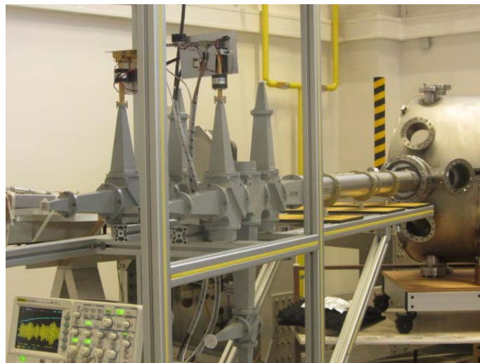
Fig. 1. Testing of the K-band reflectometer on the vacuum chamber mock-up
