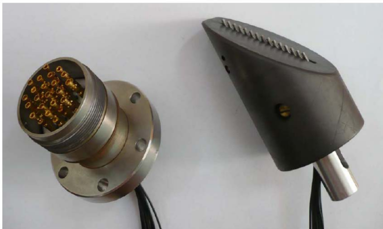
Fig.2: Photograph of the second LP array to be installed in COMPASS divertor
