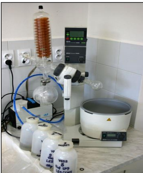
Diluted liquid samples can be preconcentrated before analysis on the vacuum rotatory evaporator . Samples are delivered in the plastic bottles, transferred into an evaporation flask and evaporated in vacuo . Concentrated sample resulting is present in a small flask connected to the apparatus.
