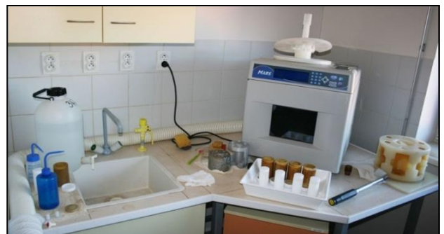
Microwave oven is not only useful in a house kitchen, but with a special teflon PTFE pressure bombs it is useful for decomposition of samples as well. Of course, the microwave power inserted on sample is far more higher than in the kitchen models.
