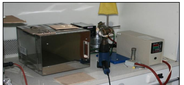
Another approach to decomposition of minerals is based on melting in resistance oven upon regulated temperature up to 1,300 °C in platinum, silver or quartz crucibles.
