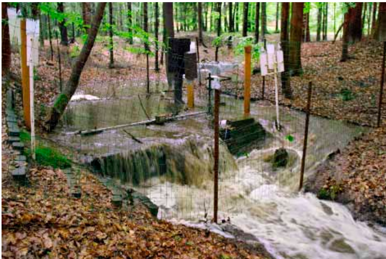
■ Fig. 11. The V-notch weir at the Lesní potok catchment on 2 nd June 2013 (2:50 P.M.) during estimated discharge of 176 \text{ l}\cdot\text{s}^{-1} ( 0.9 \text{ mm}\cdot\text{hr}^{-1} ). The daily amount of precipitation on 2 nd June 2013 reached 63.4 mm. The amount of precipitation for period 30 th May – 3 rd June 2013 summed up to 131 mm. Photo by T. Navrátil.
