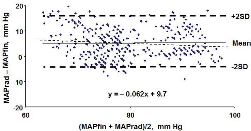
**Fig. 2.** The Bland-Altman plot for radial mean arterial pressure (MAPrad) and finger mean arterial pressure (MAPfin). Differences between MAPrad and MAPfin are plotted against the average of MAPrad and MAPfin values. The horizontal bold dashed lines represent the 95 % confidence intervals ( $\pm 2$  SD from the mean difference). The regular dashed line represents an overall linear regression.
