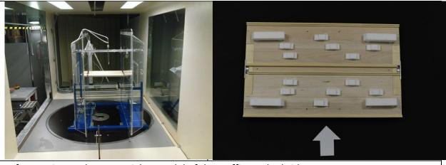
Left-Experimental set-up. Right- Model of the traffic on the bridge
