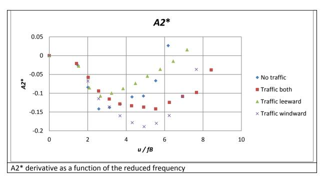
One can also observe a significant influence of traffic position on stability of bridge deck. It seems that deck without traffic is most susceptible to flutter instability, while the traffic windward is most stable one. Furthermore, deck without traffic experience the sudden loss of stability alike the case with the traffic. Also, A2\* turns positive at the same reduced velocity for traffic in both directions and traffic positioned windward.
