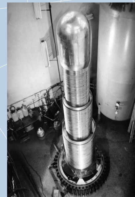
Former Van de Graaff accelerator, now part of National Technical Museum in Prague
