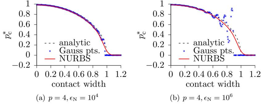
**Figure 2.** Contact pressure distribution.
