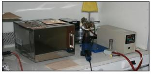
Another approach to decomposition of minerals is based on melting in resistance oven upon regulated temperature up to 1,300 °C in platinum, silver or quartz crucibles. SPECIAL EQUIPMENT AND TECHNIQUES FOR WORKUP, PREPARATION AND STUDY SAMPLES
