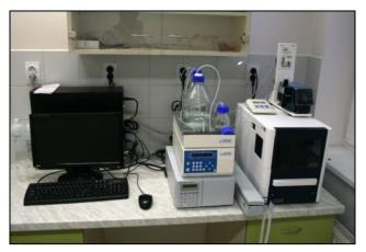
The presence and amount of nitrates, chlorides, sulfates and other anionic component is analysed on the **HPLC liquid analyser** by chromatography on anion exchanging chromatography with conductivity detection.
