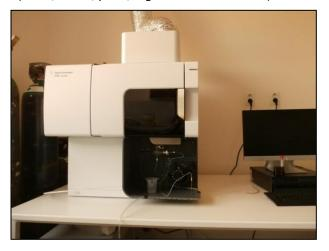
Chemical composition of samples is studied on universal multielement spectrometers in an argon plasma discharge (**ICP EOS instrument**). At temperatures about 10,000 K, chemical elements present in the sample emit visible or UV radiation, which is collected and processed. As a result, certain element is identified together with its content in the sample.
