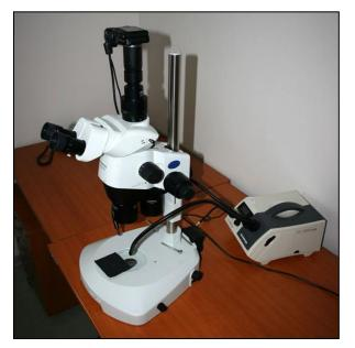
**OLYMPUS SZX 16 Optical binocular microscope** with the **CANON digital photocamera** and specialized **QuickPHOTO Micro software** and a **Deep Focus module** is used for the documentation of samples, separation of sub-samples for other methods and, of coarse, for imaging of samples and details for publications.
