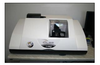
The **CILAS 1190 LD laser granulometer** is used to provide a measurement of the grain size distribution in range from 0.04 to 2,500  $\mu$ m. The measurement is based on a small amount of material and might be easily repeated. Using the different types of dispersion allows to get the picture about the primary or secondary given grain size distribution. Data can be reported in different fractions set by the user.
