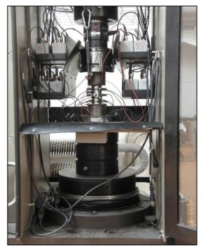
Uniaxial load frame MTS is a computercontrolled servo-hydraulic loading system specifically adjusted for long-term testing. This system allows testing of rocks in regime of controlled force or controlled deformation. Together with triaxial cell, this equipment allows simulation of pressure-temperature conditions and permeability measurements.
