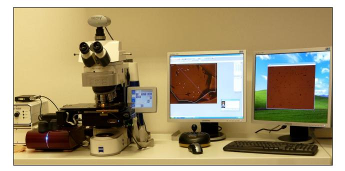
**ZEISS Imager. M1m Microscope** connected to two monitors of a computer for a fission track analysis (FTA). The Microscope is equipped with an AUTOSCAN table moving in directions x, y, z. controlled by a computer and manual joystick; two light sources using reflected and transmitted light. Another part of the microscope is a digitizing equipment for measuring lengths of specific tracks parallel to the surface of the mineral grain (i.e. confined tracks).
