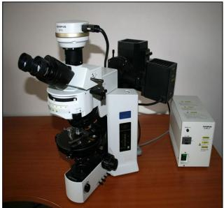
**OLYMPUS BX50 Optical polarizing microscope** with the **digital camera DP 70** and specialized **QuickPHOTO software** and a **Deep Focus module** is used for a detailed study of thin (for transmitted light) and polished (for reflected light) sections. Software enables documentation, image preparation and image analysis. The microscope is equipped also with a fluorescent source of different wavelengths.
