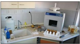
**Microwave oven** is not only useful in a house kitchen, but with a special teflon PTFE pressure bombs it is useful for decomposition of samples as well. Of course, the microwave power inserted on sample is far more higher than in the kitchen models.
