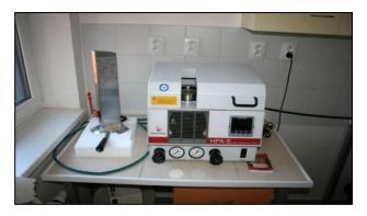
Before analysis, majority of solid samples are prepared by decomposition in acids. In the **HPA-S Anton Paar high pressure asher**, samples are dissolved at temperatures up to 300 °C and pressures up to 100 atm.
