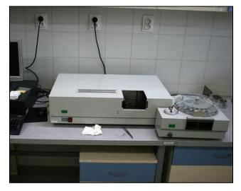
**Advanced mercury analyser** used for analysis of mercury content in solid samples. Extraordinary sensitivity (up to fractions of nanogram Hg) is reached.
