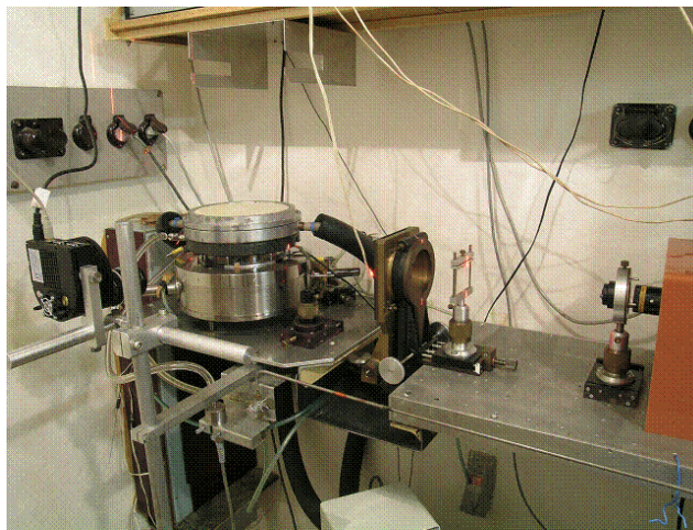
Thermal diffusion cloud chamber built at the ICPF - on the optical bench
