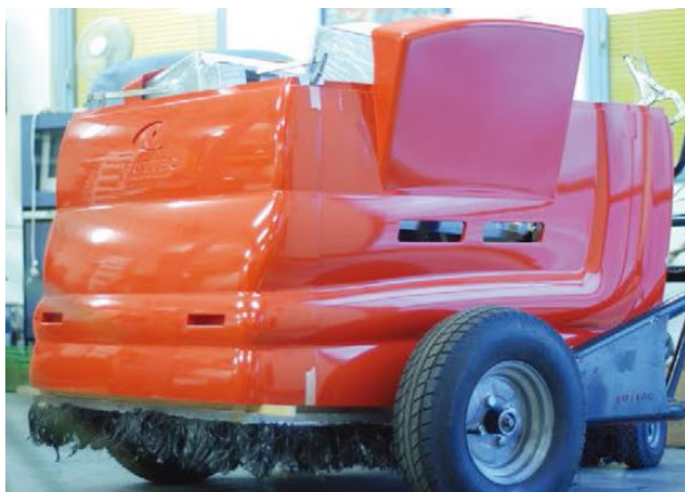
High effective machine FT3 for pothole road repairs ( http://www.iwme.cz/produkt/ )
