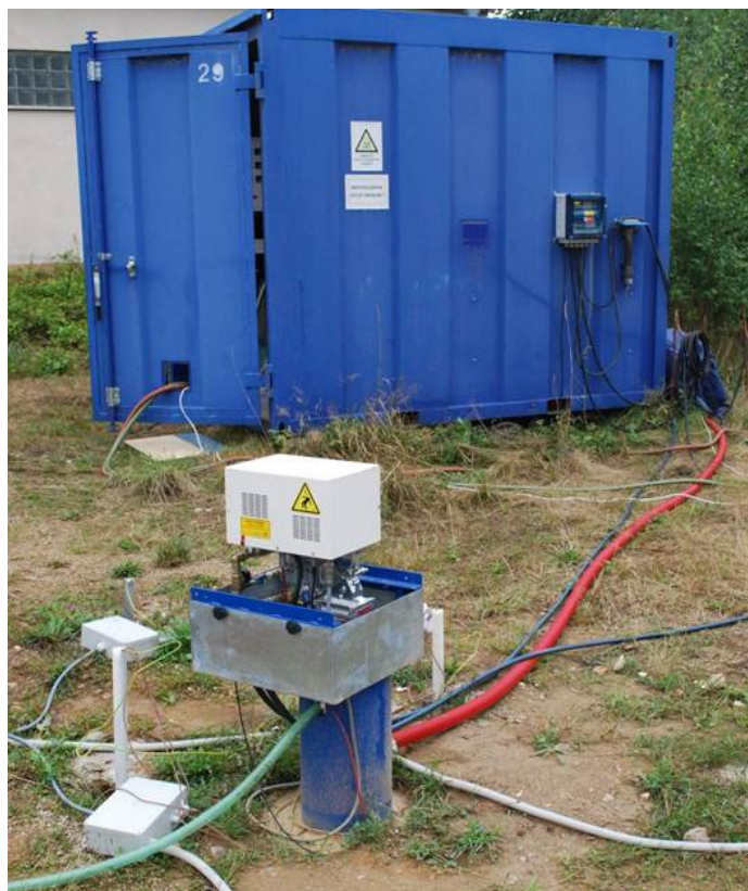
In-situ thermal desorption with use of microwaves
