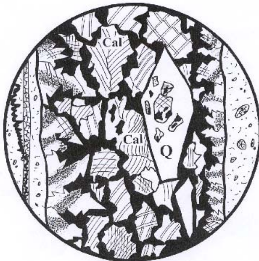
Fig A: Calcite- and bitumen-filled vein from the Lochkov Limestone, Radotín. Diameter of the circular field of view is approximately 7 mm. Note the presence of saddle-shaped dolomite crystals (Dol) along the vein margin and the intensely corroded calcite grains “floating” within the bitumen (shown in black)
