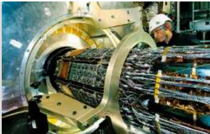
The installation of pixel subdetector into ATLAS. Michal Tomášek supervises the installation of inner pixel subdetector into the ATLAS detector at CERN
