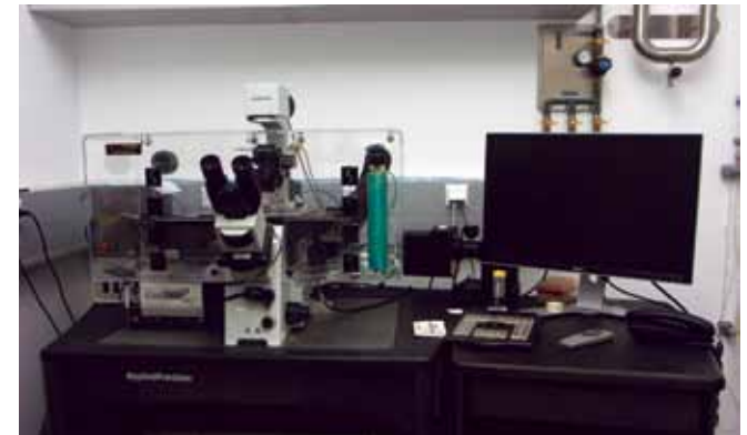
DeltaVision Core deconvolution microscope with laser photomanipulation
