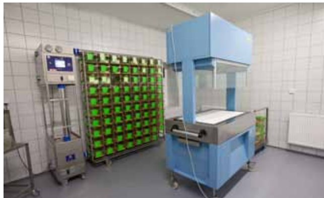
IVC rack and changing station
