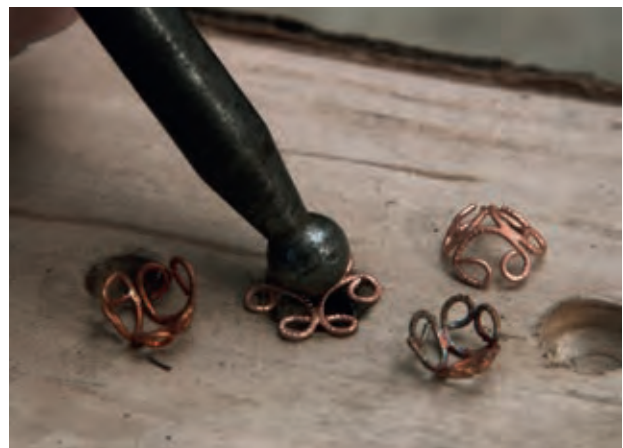
▲ Fig. 3. Shaping of filigree hemispheres.
