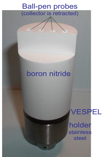
Fig.1: Four Ball-pen probes (collector diameter \varnothing 4 mm - carbon and copper, shielding tube with inner diameter \varnothing 6 mm) for the experiment on RFX. Boron nitride has a diameter \varnothing 50 mm and length 90 mm.
