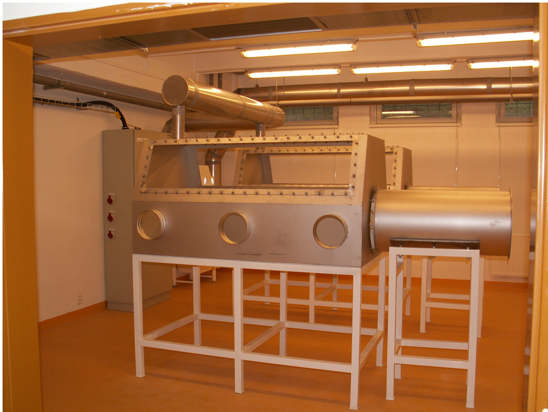
Fig. 1: A view of beryllium workplace with glove boxes for testing of Primary First Wall mock-up samples with Be armour layer
