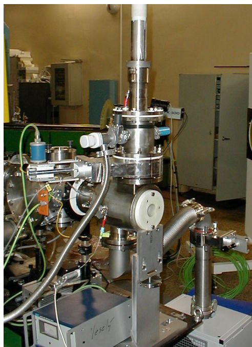
Fig.1: The target station of p\text{-}{}^7\text{Li} neutron source.
