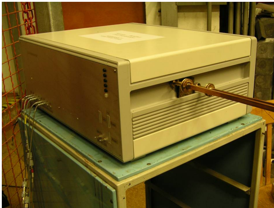
Fig. 5.2.1 Test of 2-mm interferometer on CASTOR
