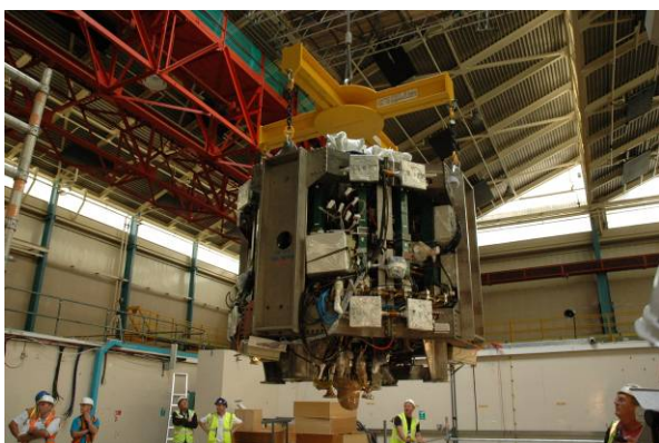
Fig. 1.2: The COMPASS-D tokamak lifting (inside the experimental hall).
