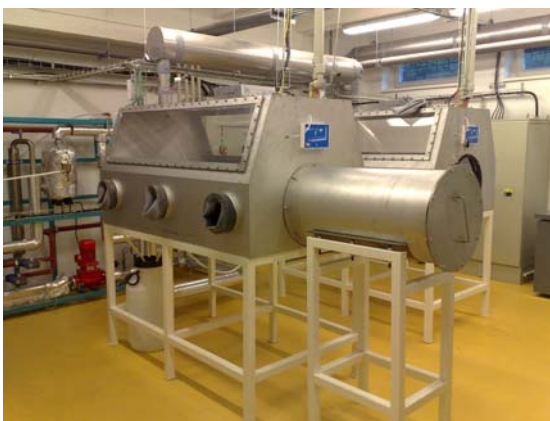
Fig 1. Laboratory for handling and manipulation with beryllium coated specimens
