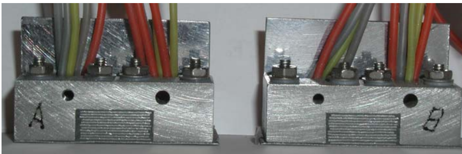
Figure 1: Picture of the 2 components of the dismantled "sandwich probe" for measuring the plasma deposition into a gap between tiles.
