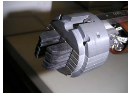
Fig. 1. Biasing carbon tips of the midplane manipulator head (without a carbon envelope) on the ASDEX-Upgrade tokamak.
