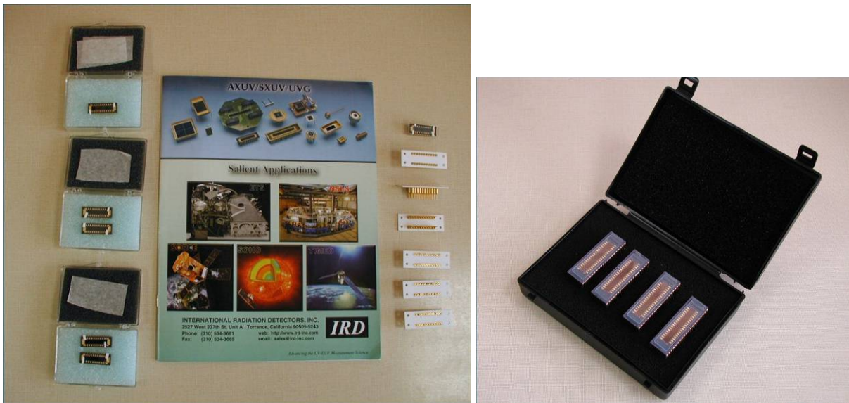
Fig. 5.3.1 On the left, there are the six AXUV20-ELM (IRD Inc.) based 20-channel arrays of fast bolometers equipped with the ceramic sockets. On the right, there are the four LD35-5T-JET-Windowless (Centronic) 35-channel arrays of the soft X-ray detectors.
