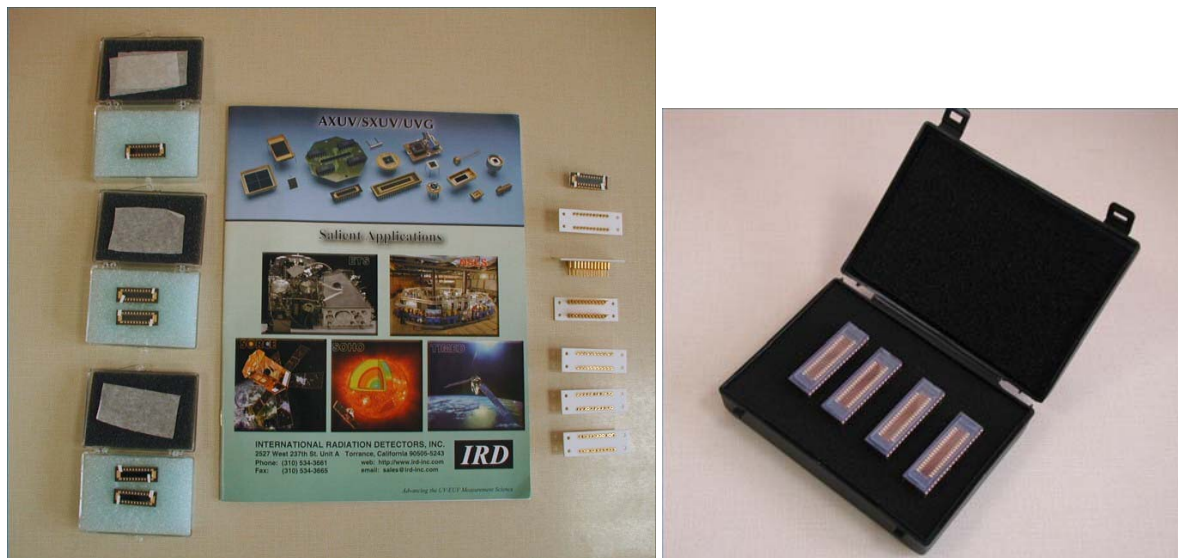
Fig.1: On the left, there are the six AXUV20-ELM (IRD Inc.) based 20-channel arrays of fast bolometers equipped with the ceramic sockets. On the right, there are the four LD35-5T-JET-Windowless (Centronic) 35-channel arrays of the soft X-ray detectors.
