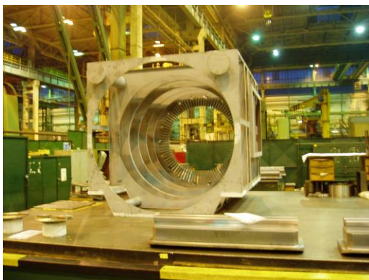
Fig. 3.1: Stator of the generator is assembled in CKD Nove Energo
