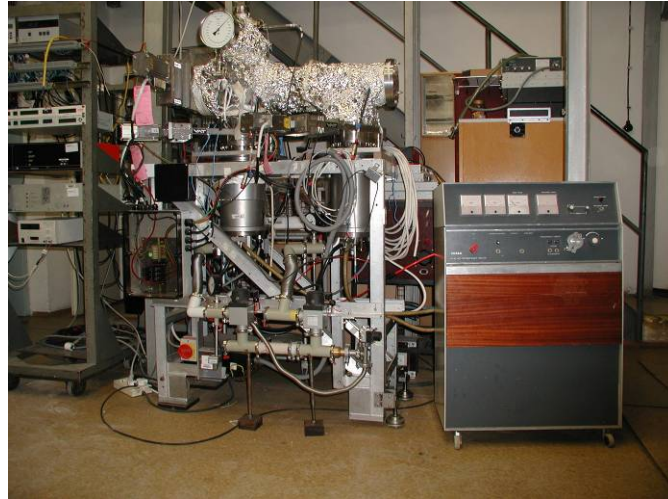
Fig. 4.1.1. The pumping system of COMPASS after testing on CASTOR
