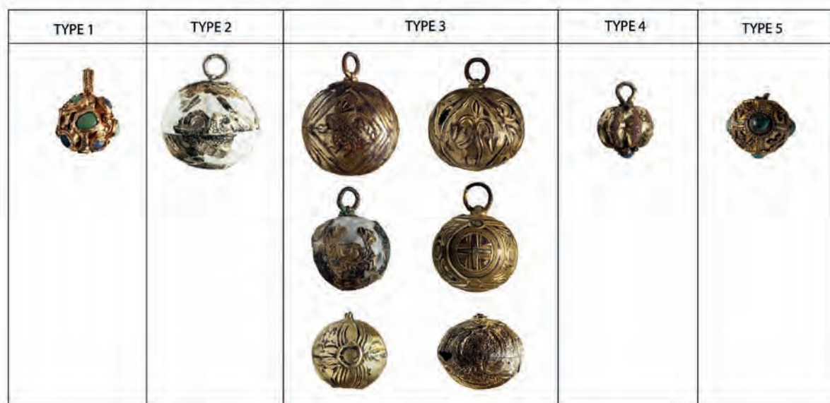
Fig. 4/1: Summarizing table of the analysed gombiky : type 1 - Au-Ag-Cu alloy, glass cabochons (H16-14), 9 different kinds of components; type 2 - Ag-Cu alloy (H115-7), 4 different kinds of components; type 3 - gilded copper alloys (H84-1, H115-8, H104-3, H108-2, H104-4, H99-5), 3 to 4 different kinds of components; type 4 - gilded copper alloy, glass cabochons (H74B-2), 6 different kinds of components; type 5 - gilded copper alloys, glass cabochons (H53-14), 8 different kinds of components.
