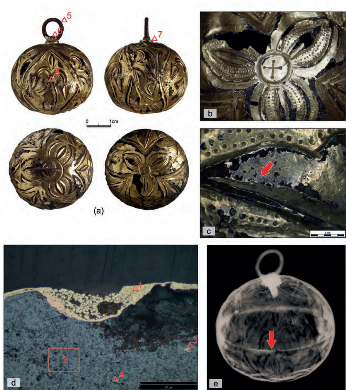
Fig. 4/7: Gombík H108-2: a - general view of the gombík (photo J. Sobek); b - detail of the cross on the bottom of the gombík (photo E. Ottenwelter); c - silvery and tarnished area under worn gilding layer (photo E. Ottenwelter); d - polished, unetched cross-section of gombík H108-1 under optical microscopy (photo E. Ottenwelter); e - X-radiograph of the gombík (D. Perlík).
