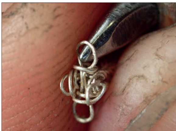
Obr. 6/321: Poté je kroužek urovnán tak, aby přechýlil na obou stranách stejně. Fig. 6/321: Subsequently, the small loop is arranged so that it equally protrudes on both sides.
