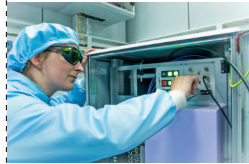
Operation of the Hydrogen maser – a radiofrequency reference
