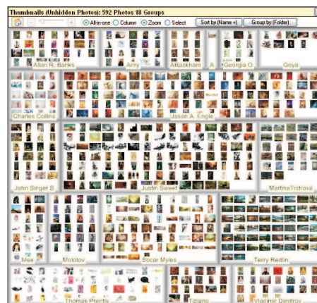
Figure 7: A gallery of pictures displayed in a quantum tree-map with Photomesa image browser. Each partition represents a folder. Here, the algorithm is optimised to use available space as efficiently as possible, while enforcing rectangular partitioning.
