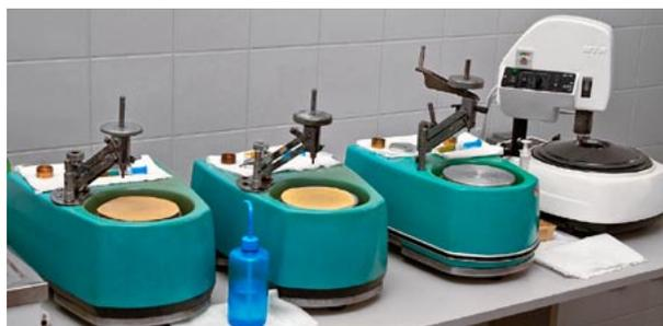
■ **Fig. 10.** Grinding machines with diamond plated wheel Montasupal and custom-made grinding machines with wheels for loose abrasive powder. Photo by R. Skála.
