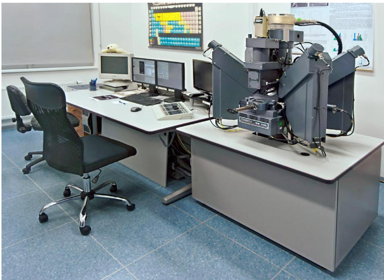
■ Fig. 8. CAMECA SX-100 electron probe microanalyzer with four wave-dispersive crystal spectrometers. Photo by R. Skála.
