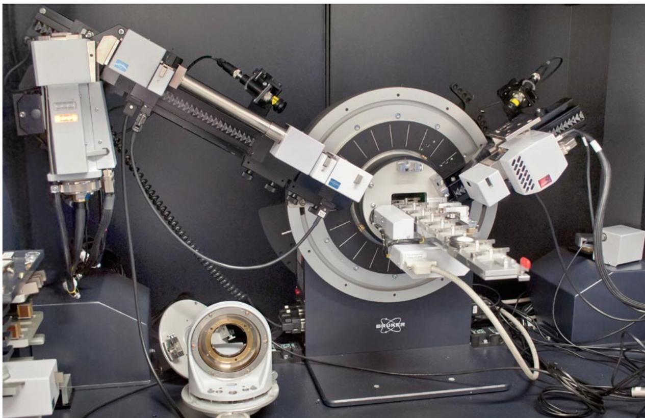
■ **Fig. 9.** Bruker D-8 DISCOVER multi-purpose X-ray powder diffractometer with installed Flipstick automatic sample changer. Photo by R. Skála.
