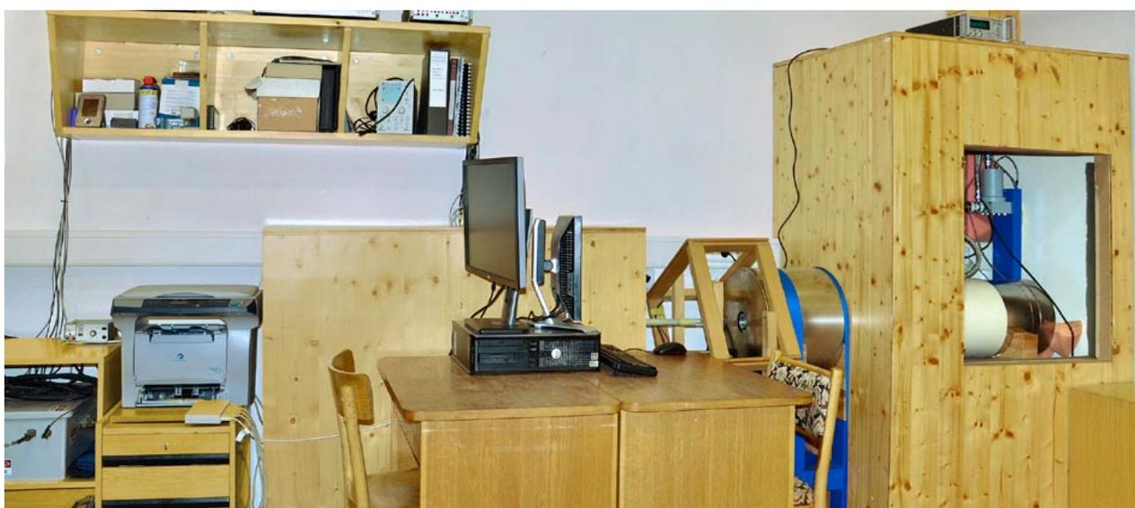
■ **Fig. 12.** An 2G 755 4K Superconducting Rock Magnetometer: an automatic precise magnetometer equipped with AF demagnetizer. Photo by P. Schnabl.
