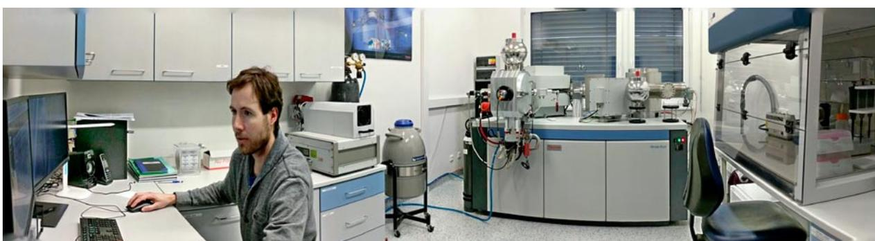
■ Fig. 6. Thermal ionization mass spectrometer (TIMS). Photo by M. Svojtka.
