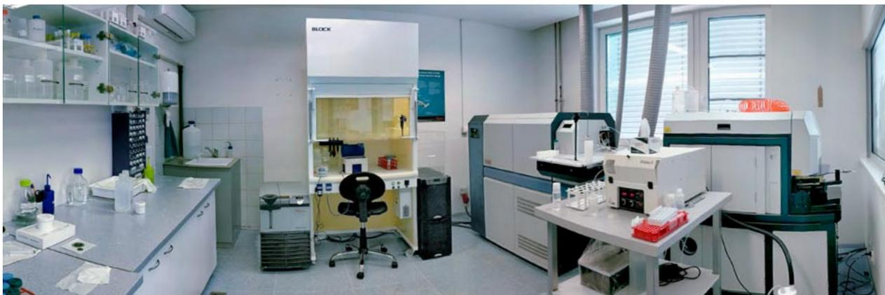
■ Fig. 5. Magnetic sector field ICP-MS coupled with an excimer laser ablation system. Photo by M. Svojtka.
