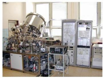
sensitivity at low detection angles. The spectrometer can be operated in transmission, spatial and angular mode.
