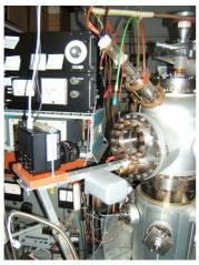
The UHV apparatus for FEM, FIM. Evaporation sources mounted on a rotatable x-y-z manipulator enable deposition of different metals or oxides onto field emission tip. The field emission and field ion images can be captured by a astronomical CCD camera with very high quantum efficiency, 16-bit digitization, low noise, fast USB interface and ability to integrate light during long exposures.
