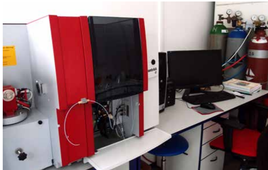
High-Resolution Continuum Source Atomic Absorption Spectrometer ContrAA 700 (Jena Zeiss) with possibility to change quickly from flame technology to graphite furnace technology
