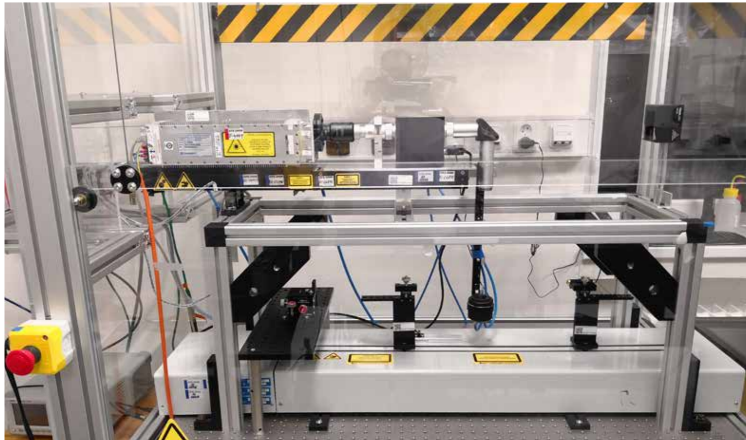
CO 2 laser for the preparation of special fiber components
