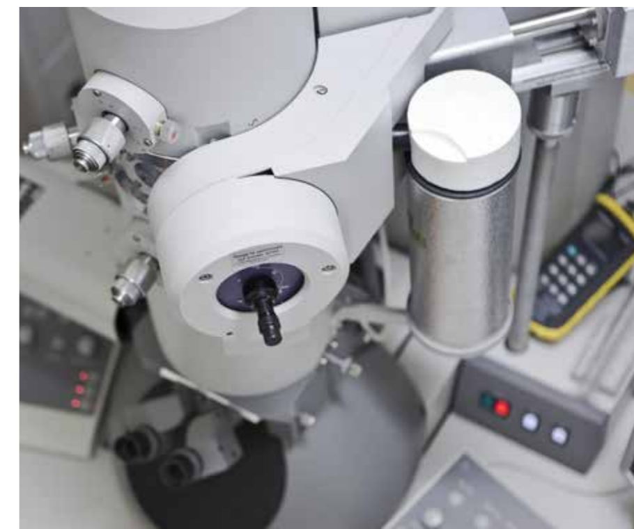
Transmission electron microscope for cryoscopic measurements
