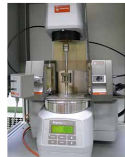
Rotational rheometer Anton Paar MCR 501 with an oven up to 400 °C and in-built camera
