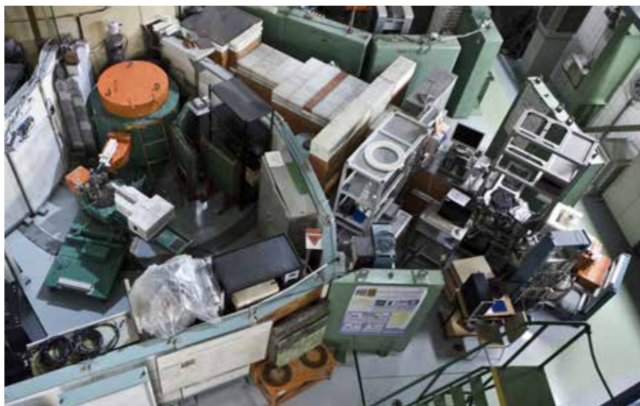
An SPN-100 neutron diffractometer for scanning tension in materials (left) and analytical methods for neutron in-depth profiling and prompt gamma activation analysis (right) on neutron beams in a research reactor
