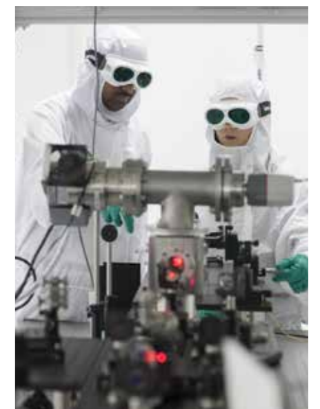
Micro-chip laser setup for material characterization and development of compact lasers.
