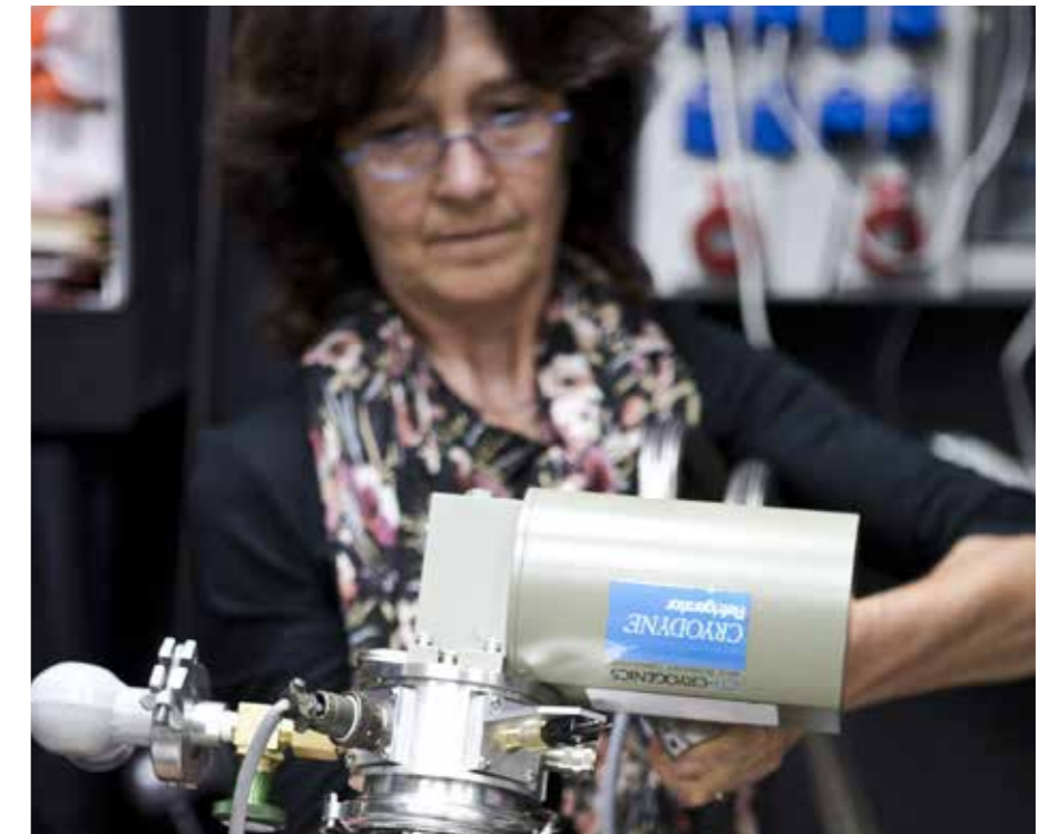
The cryostat head of a Janis closed-cycle refrigerator
