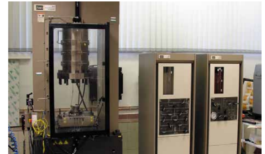
Multipurpose servo-hydraulic loading system with triaxial cell
