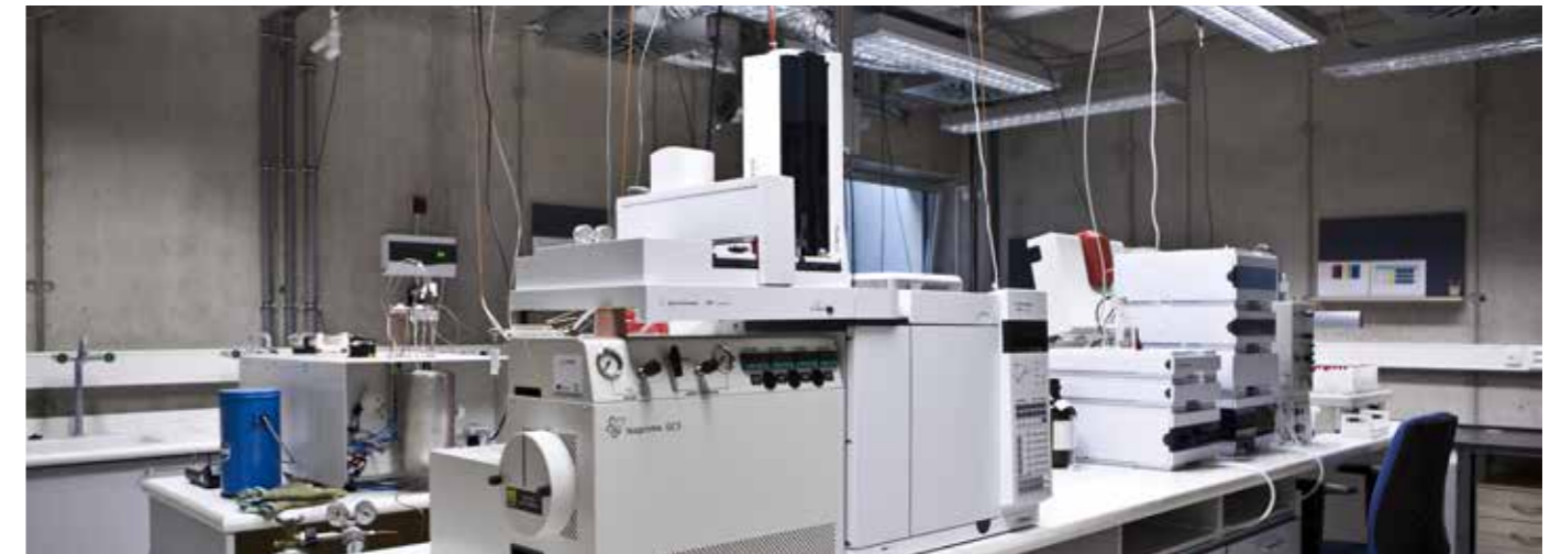
The isotope laboratory is used to evaluate the natural discrimination of stable isotopes C, N, H, O. The discrimination is, for example, an indicator of the efficiency of plant's utilization of water or the type of photosynthetic metabolism
