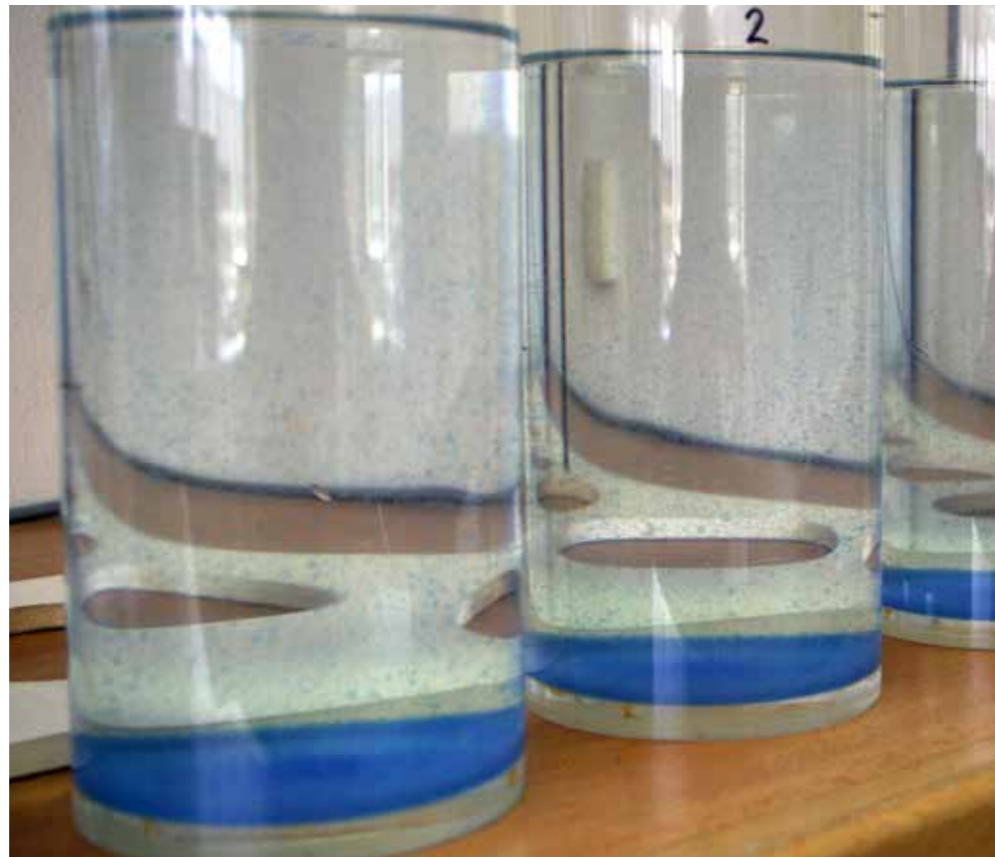
Jar test – Optimization of coagulation
