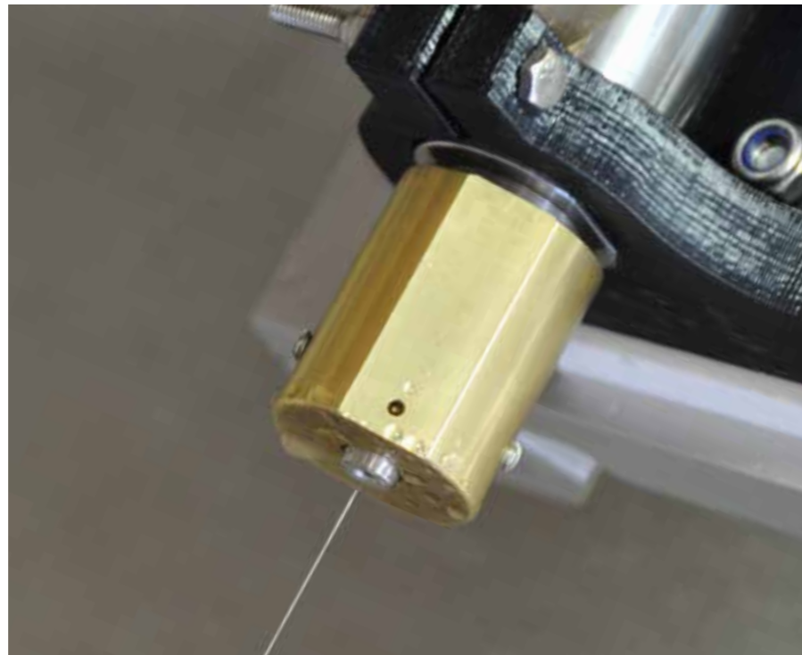
Prototype of a water jet cutting head for medical applications
