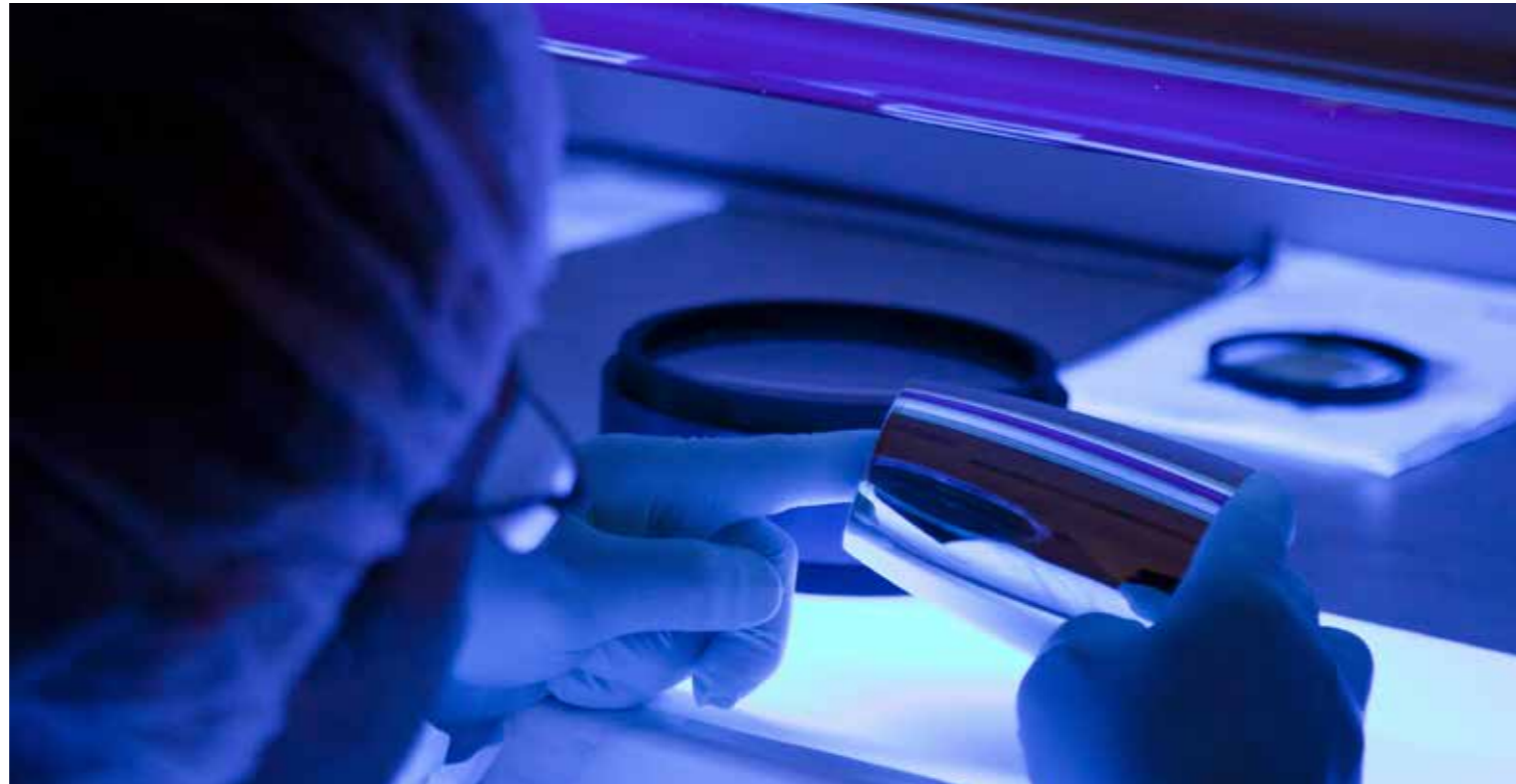
Output visual inspection of the mandrel of an X-ray objective
