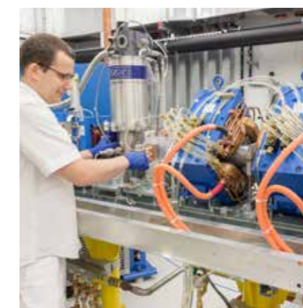
Ionto-optical beam-line of the TR-24 cyclotron
