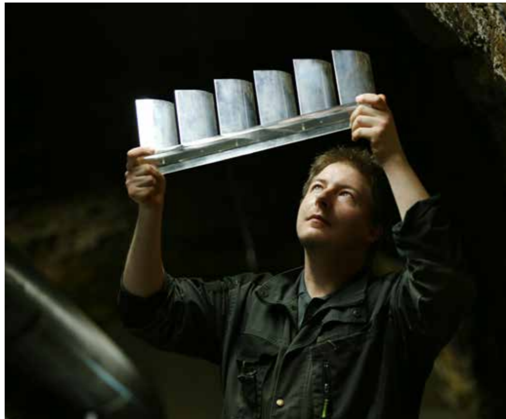
Technician Antonín Zajíček inspects the blade cascade model before mounting into the aerodynamic tunnel
