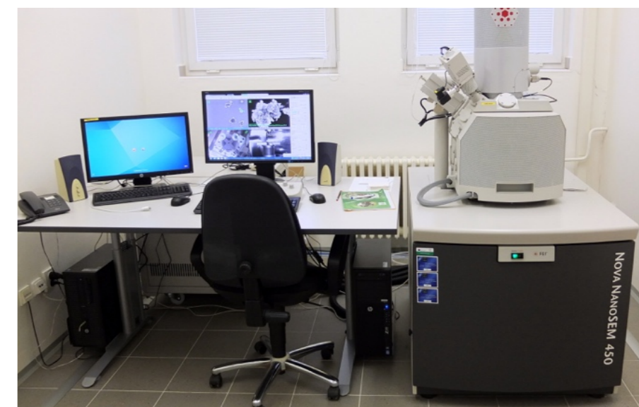
HRSEM FEI NanoSEM 450 (High-Resolution Scanning Electron Microscope)
