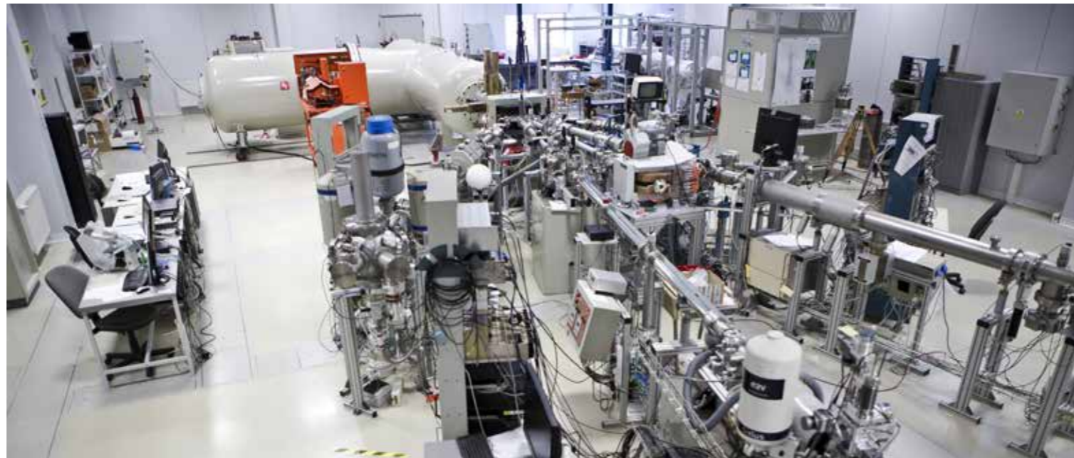
Laboratory of Tandetron – a view of beam lines with end target chambers for ion analytical methods'
