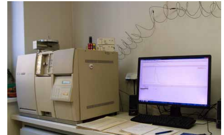
Elemental Analyzer NC 2500 (Carlo Erba) used for determination of total carbon and nitrogen
