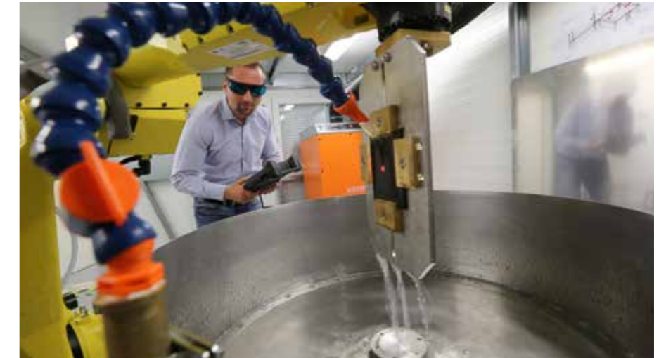
Processing station for laser driven material hardening and maintenance life-time improvement.
