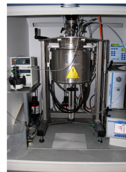
Reactor for liquid phase nanomaterial synthesis and testing catalysts and kinetic measurements
