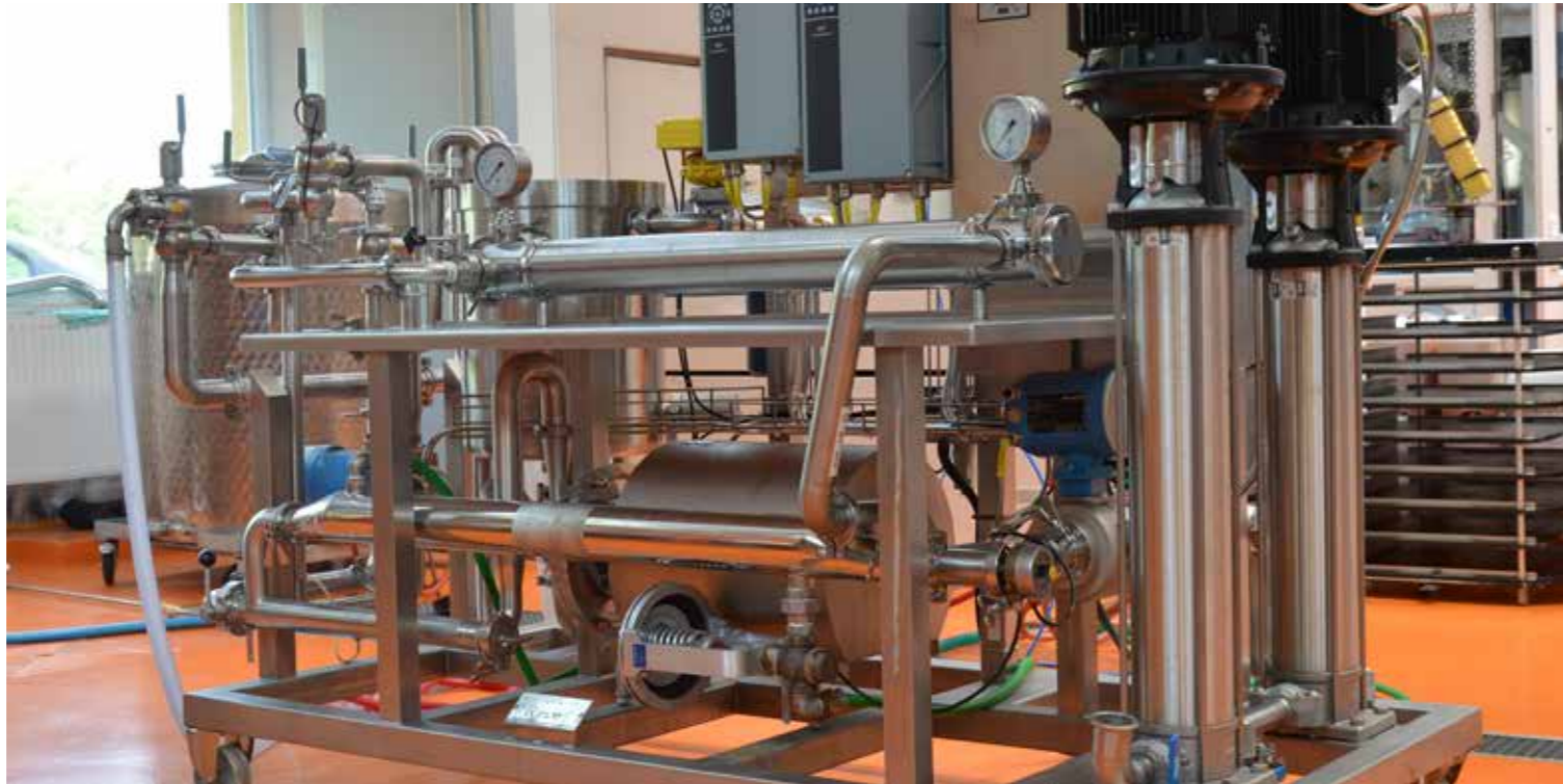
Cross-flow filtration: universal unit Alfa Laval M39/M3.8 for microfiltration, ultrafiltration,
