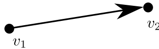
Figure 3.8: Global orientation of edge v_1v_2 in the physical mesh. Example of situation where i(v_1) < i(v_2) and therefore the orientation is from v_1 to v_2 .
