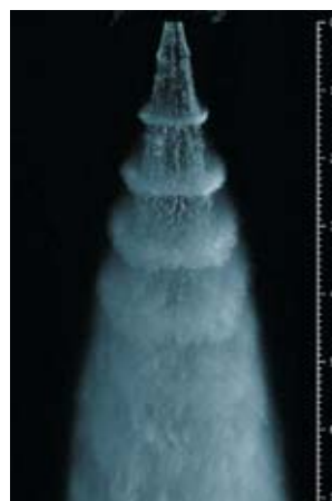
Pulsing fan water generated at 20MPa. The scale represents the stand-off distance of in mm. (photo: Archives of the Institute of Geonics )
