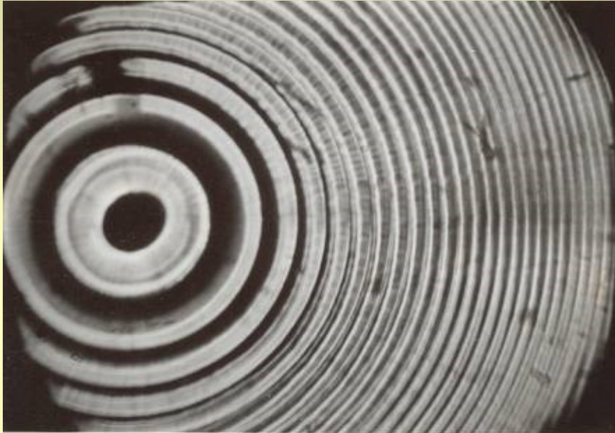
Microphoto of cross section of produced preform
